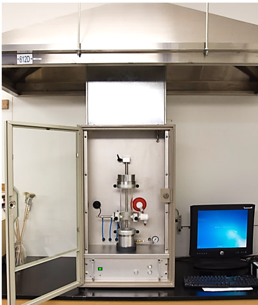
Figure 7 : Minimum Ignition Energy Device (MIKE3) [33]
