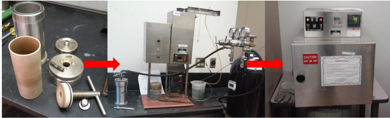
Figure 54 – Setup for HT/HP Solubility Tests
