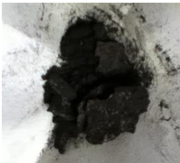
Figure 48 – HT/HP Mud Acid Solubility of the Scale Sample
