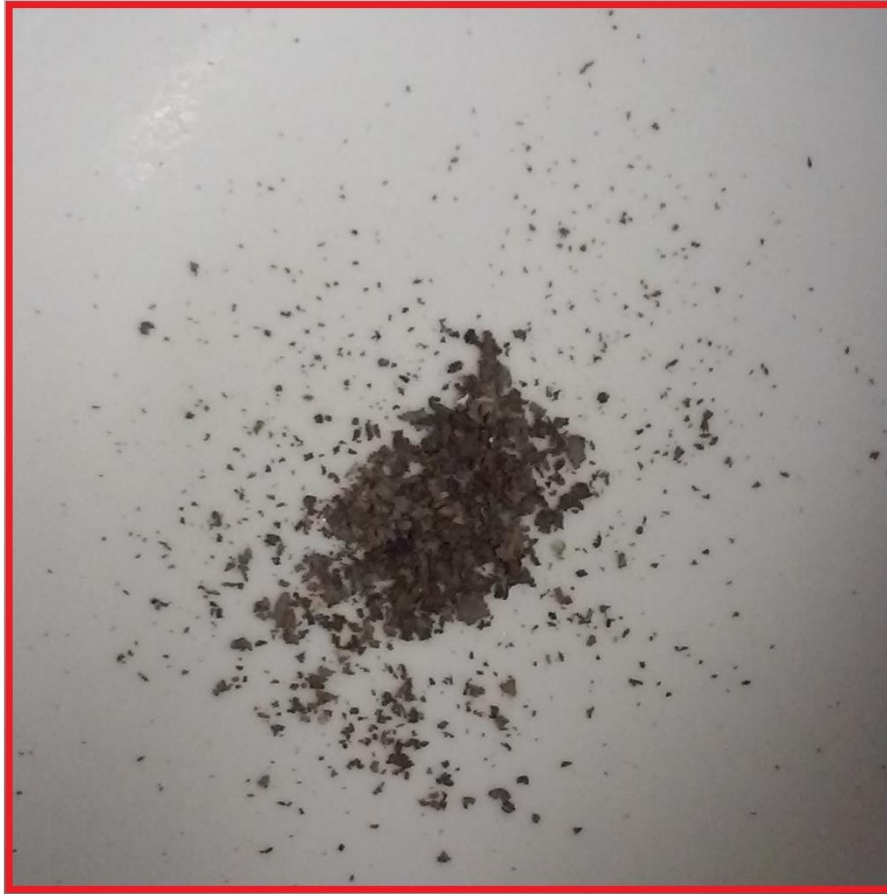
Figure 40 – Solid Precipitation Material Collected from the Sandpack with Illite
