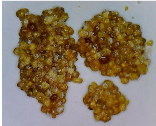
Figure 3.2 Large agglomerates of resin-coated sand proppant after testing under stress.
