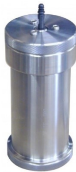
Figure 2.12 OFITE stainless steel HP/HT aging cell with a non-stick Teflon liner
