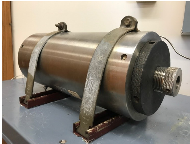
Figure 2.7 High-pressure cylindrical core holder with a Hassler rubber sleeve.
