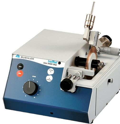
Figure 2.4 IsoMet BUHLER high precision cutter used to cut the core samples.
