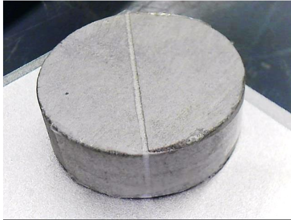
Figure 2.6 An image of the experimental propped fracture model. Reprinted from SPE-191240-MS.
