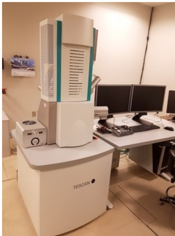
Figure 2.13 VEGA3 TESCAN scanning electron microscopy with an energy dispersive X-ray spectroscopy.
