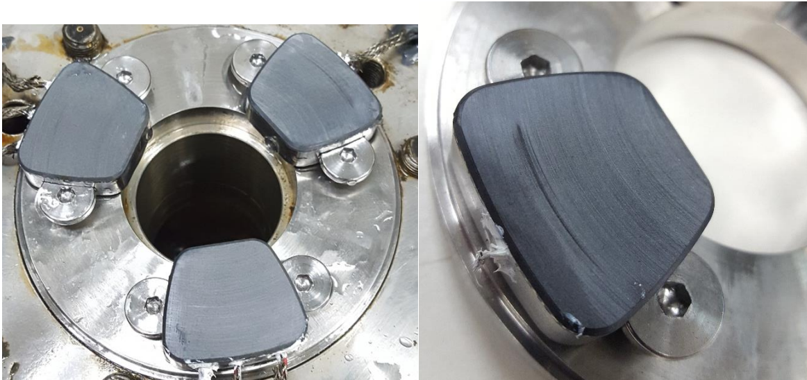
Figure 47 PEEK bearing after operating at 350 psi (2.41 MPa) at 3600 RPM. Close up view on the right
