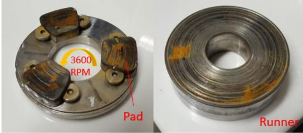
Figure 38 Left: WC bearing post 3600 RPM static test. Right: steel runner after testing. Source of rust is the 17-4 PH stainless steel runner.
