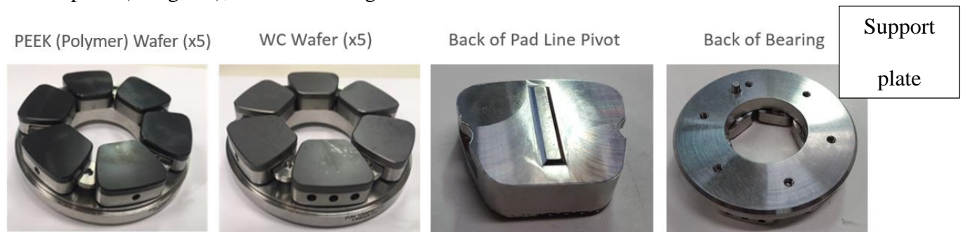
Figure 18 Picture of PEEK and WC wafer test bearings
