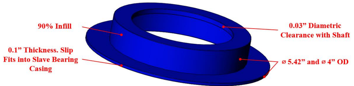
Figure 58 Plastic splash guard model and notable features
