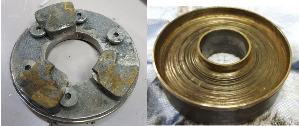
Figure 51 WC bearing (left) and runner (right) after the wear test
