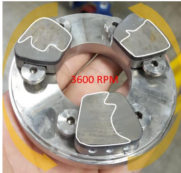
Figure 39 Direction of rotation shown in yellow vs wear pattern for WC bearing. White region denotes leading edge.
