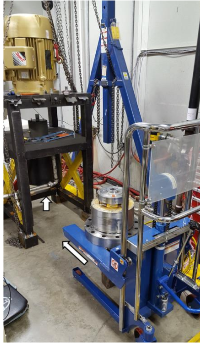
Figure 13 Test bearing assembly. The bottom assembly is lowered on the lift and pushed under the structure where it is raised into the test rig
