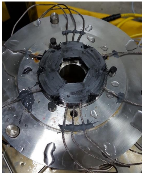
Figure 22 PEEK bearing damaged during testing. Only 100 psi of unit load was applied.
