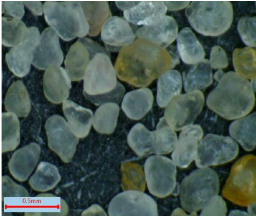
Figure 3.11 Magnification of Schlumberger Brown 4070 Mesh
