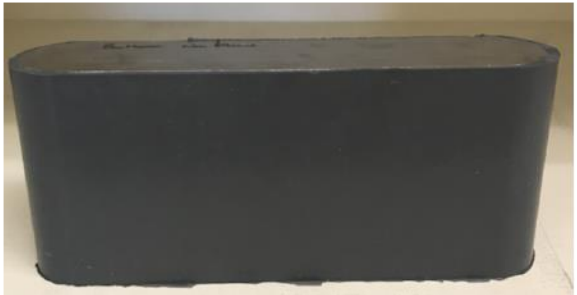
Figure 2.5 Steel plate with rubber epoxy surface applied to outside surface (Wylie, 2018)
