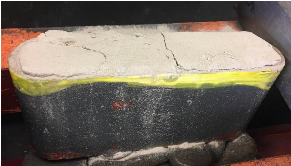
Figure 3.38 100 Mesh Keetac Sample #1 after conductivity test
