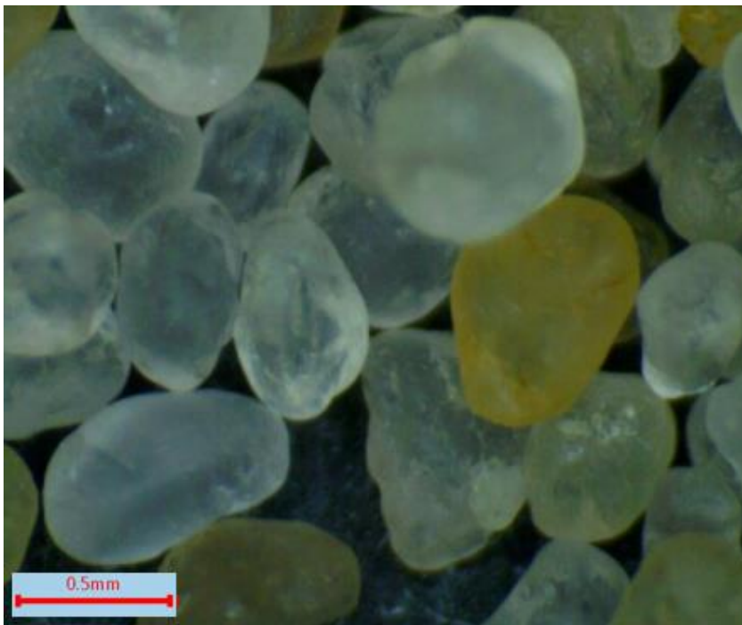
Figure 3.5 Magnification of Schlumberger Brown 3050 Mesh
