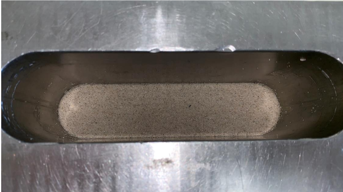
Figure 2.9 Top view of 1/4" Proppant Pack evenly distributed
