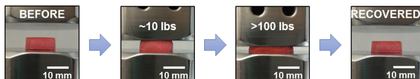
Figure 4-1. Photo series of the compression and recovery of thermoresponsive DN hydrogels under a load of >100 lbs.
