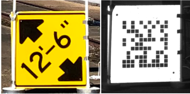
Figure 3.2: Sign as seen in visible spectrum, left, and infrared light, right
