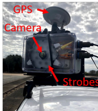
Figure 3.10: Camera apparatus mounted on vehicle used for experiment
