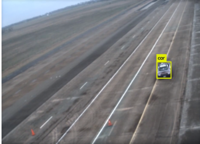
Figure 2.3: Bounding box around vehicle as detected by an MSSP
