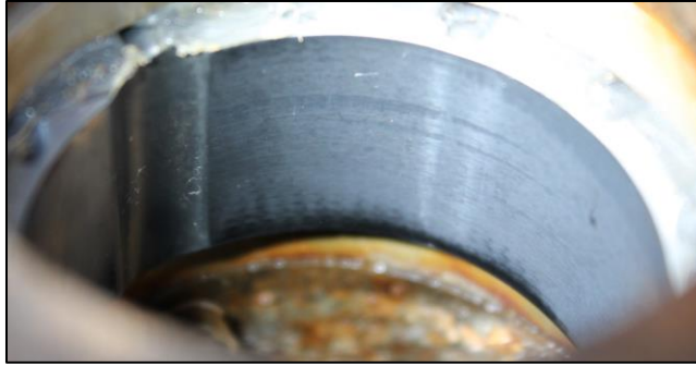
Figure 6- 10 Seal polishing after 50 hours of operation from SiC test no. 4 with an initial radial clearance of 15 \mu\text{m}
