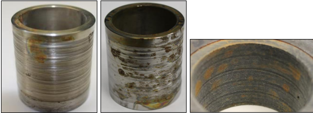
a) 30% GVF sleeve (test 3) b) 60% GVF sleeve (test 5) c) 60% GVF seal (test 5)
