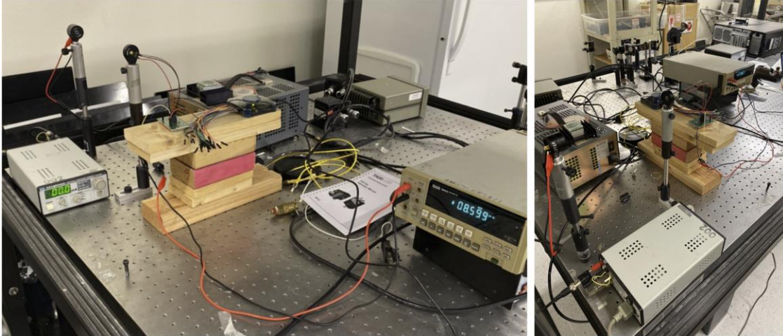
Figure 1.6.20: Actual Experimental Setup for PD Operating Circuit
