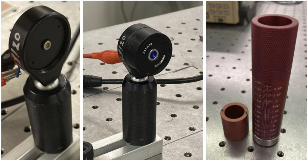
Figure 1.6.11: VCSEL and Collimating Lens Hardware Setup
