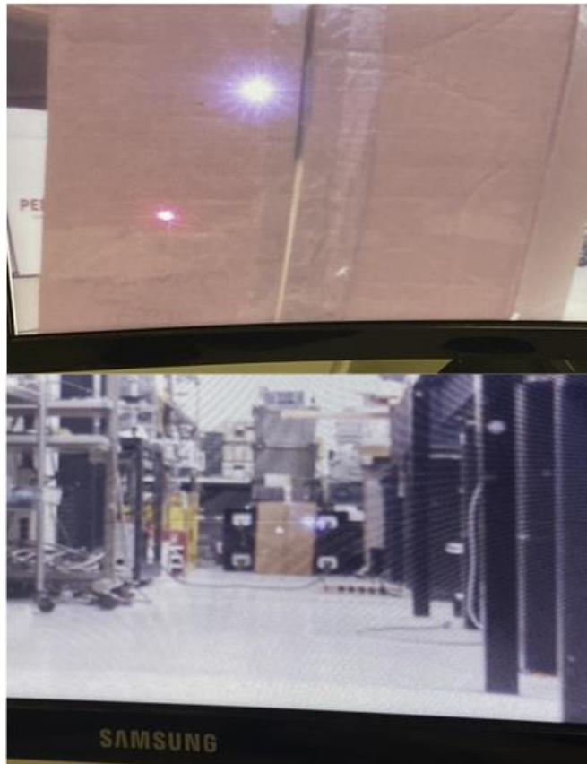
Figure 3.5.10: Test Laser Diode and VCSEL Diode Beam Spots Seen by the Stationary Module's Raspberry Pi Camera at Distances of One Meter (Top) and Ten Meters (Bottom)
