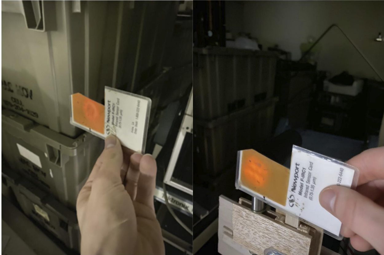
Figure 3.3.1: Comparison of Old vs New Collimated VCSEL Beam Pattern at 10 Meters
