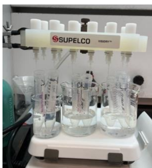
Figure D.2. Nitrogen drydown process. Elute tubes containing elute and residual methanol were placed in beakers of water and set upon a heater. To quickly evaporate the methanol, gently blowing nitrogen was introduced.
