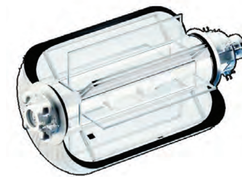
Figure 5.B - Deployable Frame (DF) deployment
