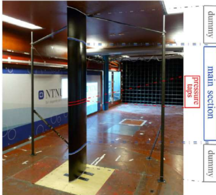
Figure 3.2: Setup of the NREL S826 airfoil experiment, adopted from [2].
