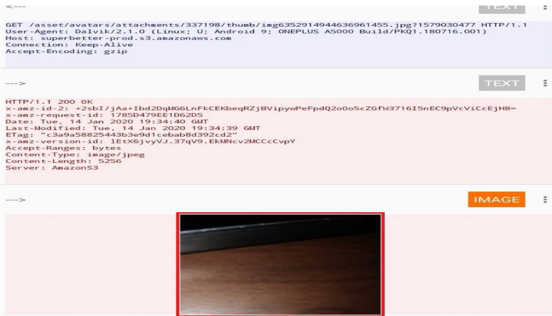
Figure 5.6: SuperBetter : Traffic captured through pcap shows Unencrypted Image
