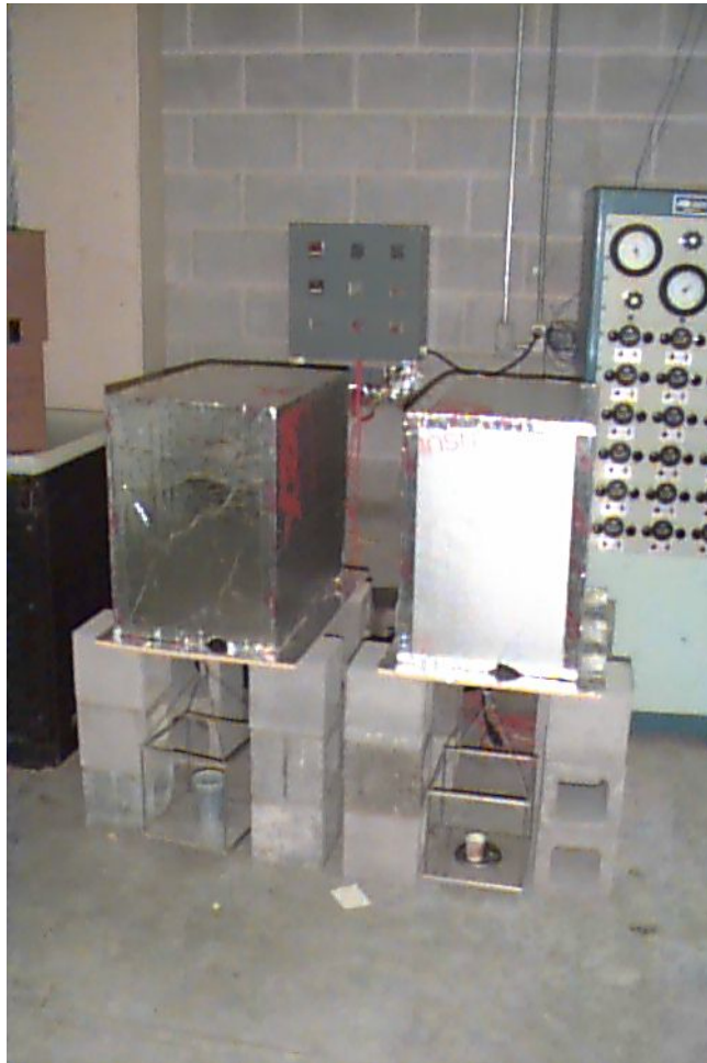
Figure 3: Creep stands with environmental chamber enclosures used for testing PVC tensile specimens.
