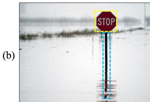
Figure IV-19 Demonstration of challenging cases in post-flood photos: (a) multiple detections (base photo courtesy of Steve Zumwalt/FEMA), and (b) reflection in water (base photo courtesy of TSGT Mike Moore, USAF).
