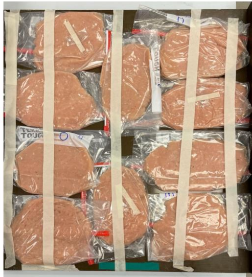
Figure 2.1: Orientation and array of ground chicken pouches for electron beam device processing/irradiation to pasteurize chicken meat prior to inoculation with microorganisms.
