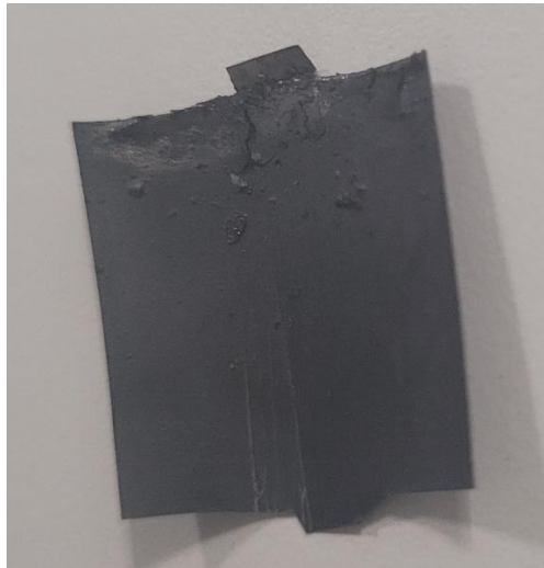
Figure 15 Mobil DTE 732 test strip with coke.
