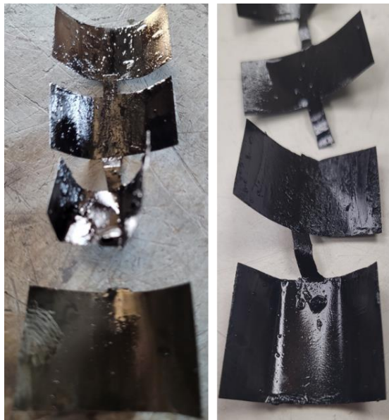
Figure 18 Two samples of SAE 20W-50 motor oil test strips with coke from 475 °C run.
