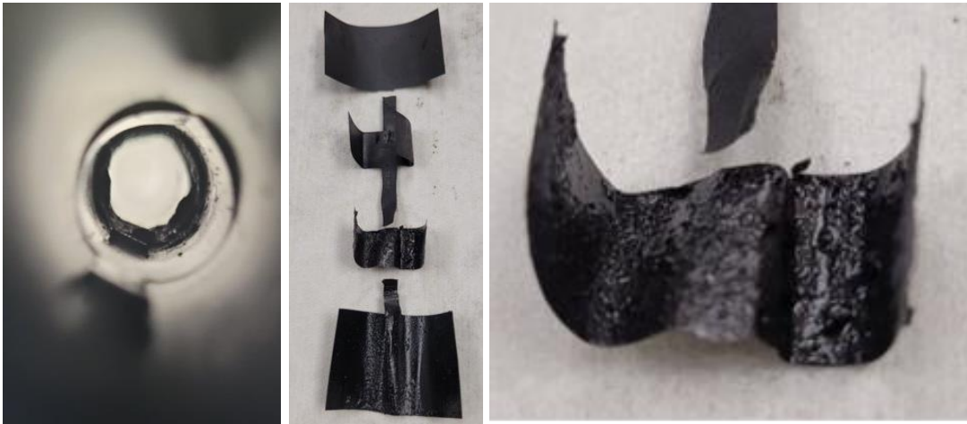
Figure 13 Flushing/rust preventative oil test strip with coke.
