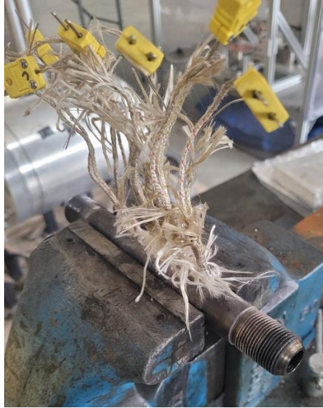
Figure 8 Test section with thermocouples.
