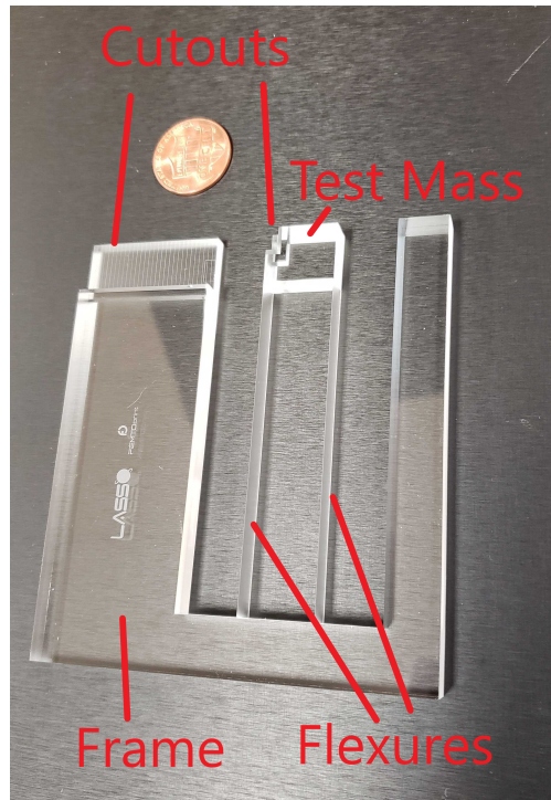
Figure 4.1: A diagram of our 5 Hz resonator. A penny is added for reference.
