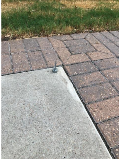
Figure 10: The 400 \mu\text{Ci} Cs-137 source placed on a concrete walkway used for testing the mobile system under working conditions.
