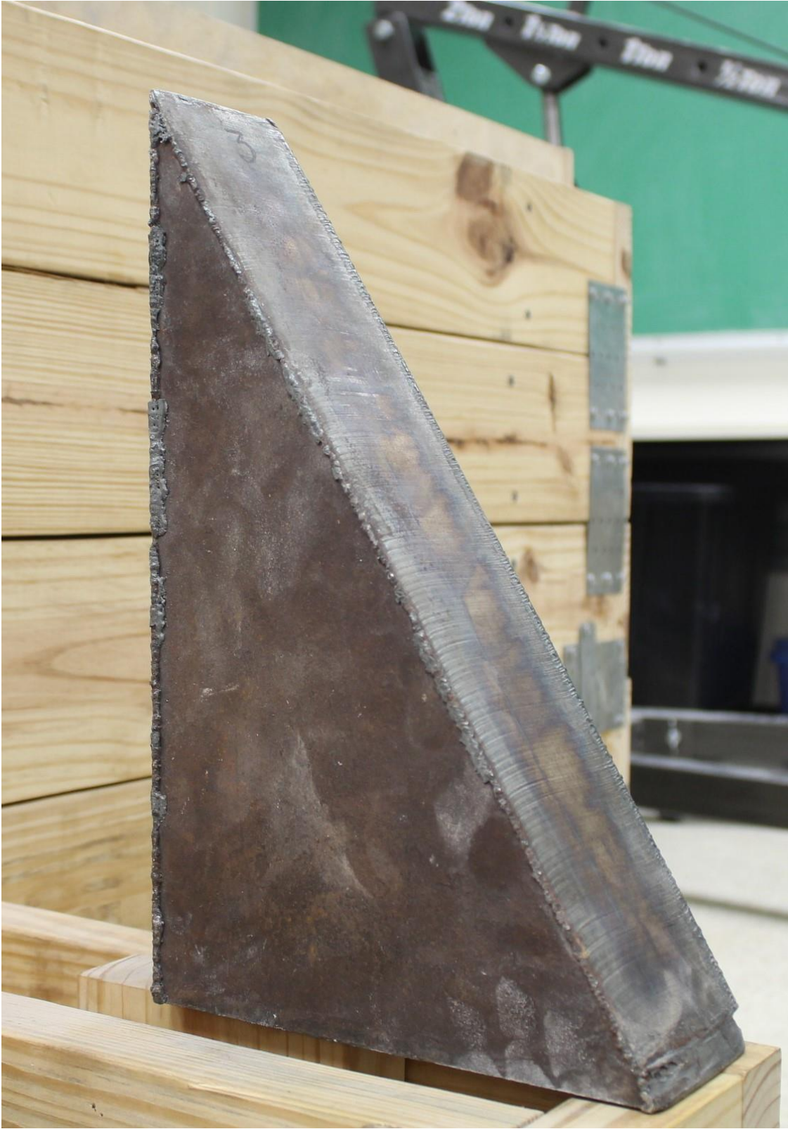
Figure 13: Picture of the Steel Weight Being Used for the Load
