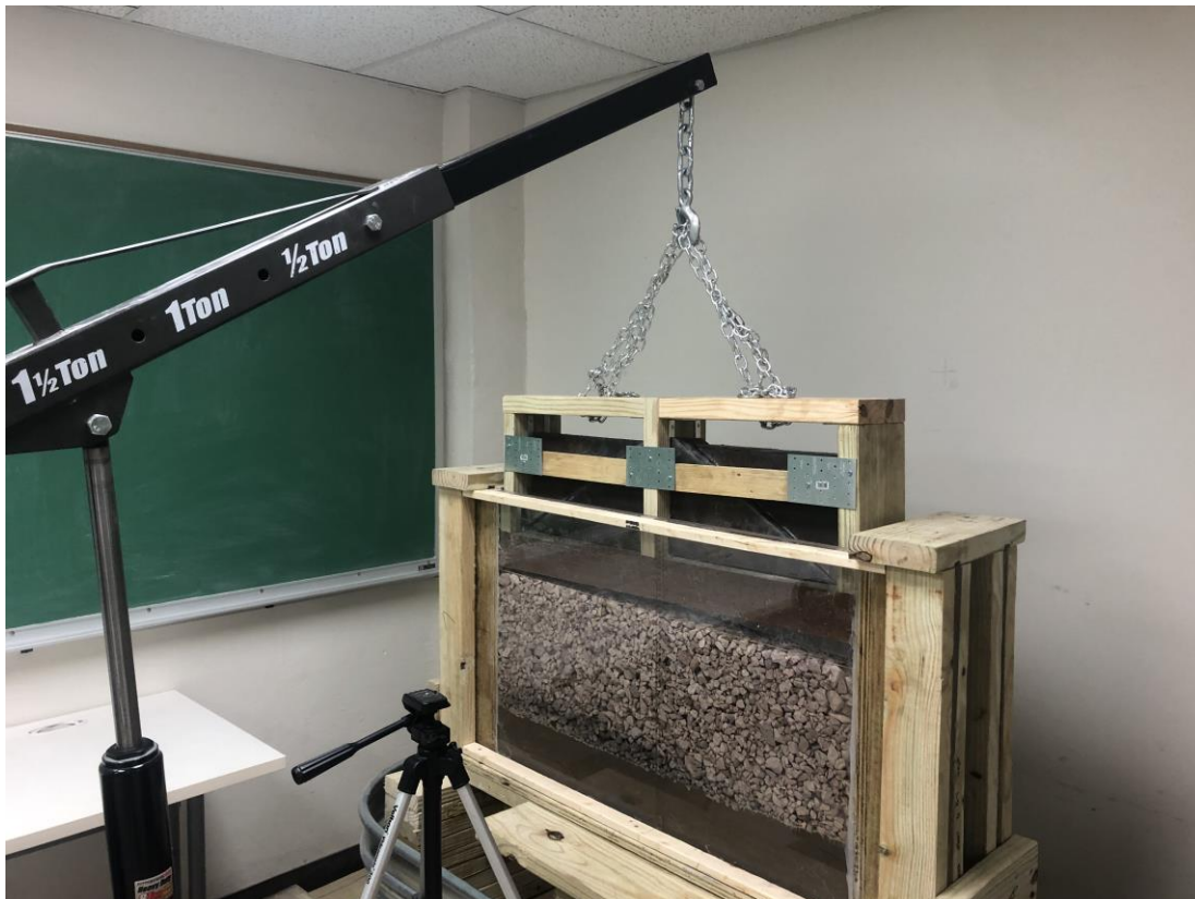
Figure 12: Picture Showing the Full Experimental Setup of the Foundation Box with the Load
