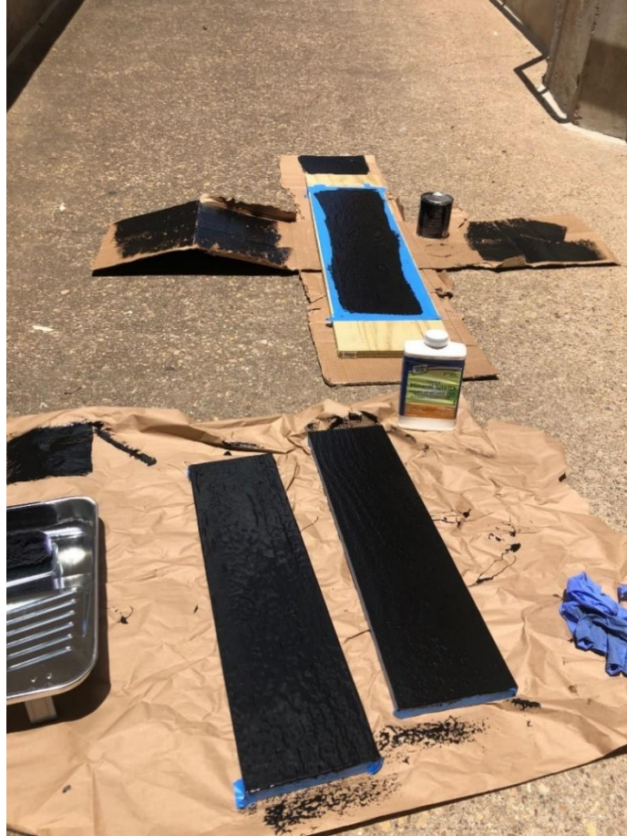
Figure 8: Flex Seal Application on Interior Side and Bottom Panels
