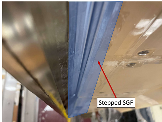
(a) Stepped SGF installed on 1/16th scale HL-CRM wing
