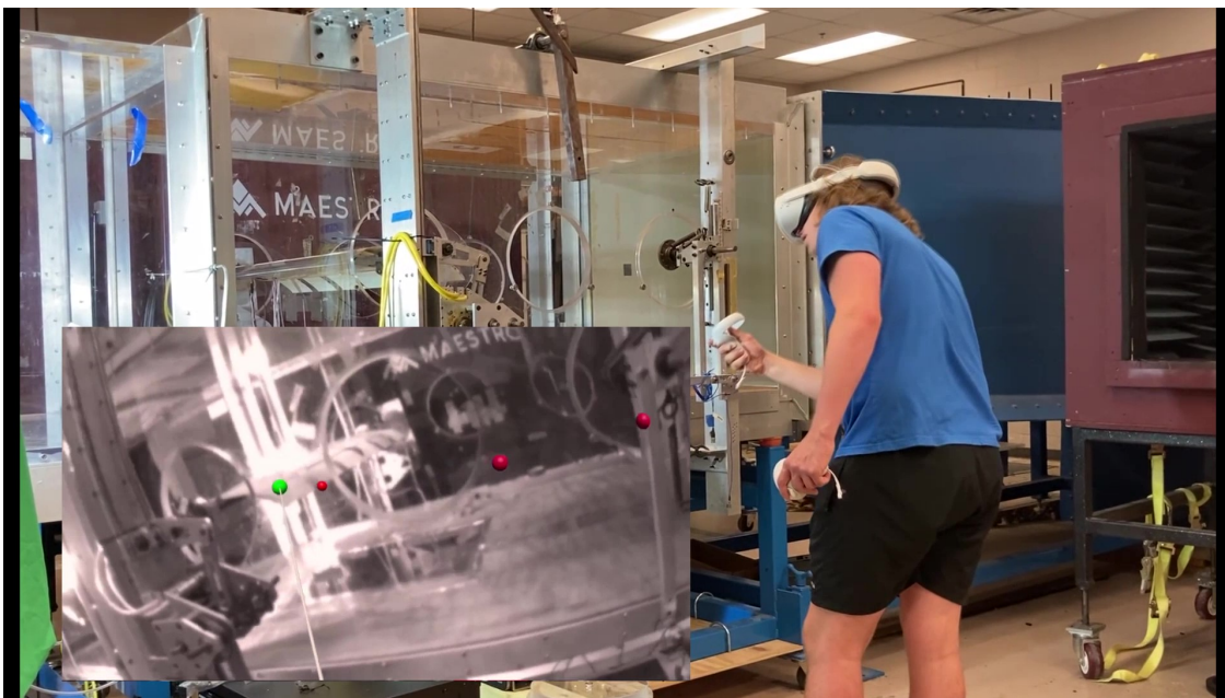
Figure 1.7: Example of a student utilizing the mixed reality toolkit to visualize flow particles while standing next to a low speed wind tunnel test section. The grayscale insert shows the view the student is seeing with the headset, with the flow particles highlighted in red.
