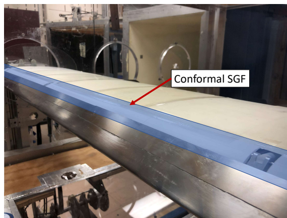
(b) Conformal SGF installed on 1/16th scale HL-CRM wing
