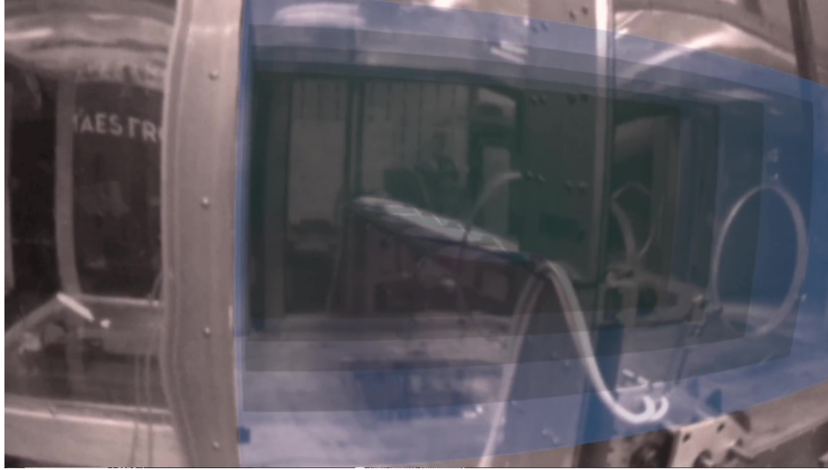
Figure 5.1: An example mixed reality object (transparent blue) aligned with an experimental test article (section spanning wing) inside of the 4 ft. by 3 ft. wind tunnel using the Oculus Quest 2.
