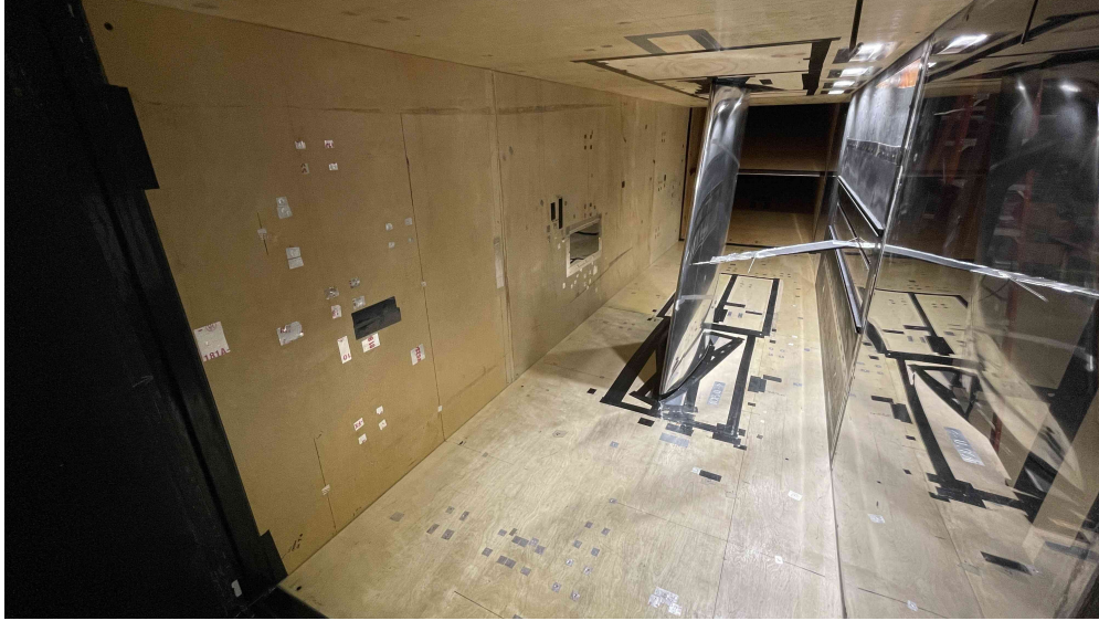
Figure 6.9: The KSWT test section including the X207.LS and the traverse system. The wing is shown at sweep \Lambda = 25^\circ and pitch \alpha = -5.5^\circ . In the top right is the temperature probe used for the Reynolds-number controller and the freestream pitot tube. Reprinted from [119].
