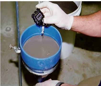
Figure 5: Fill Flow Cone to the Specified Level and have Stopwatch Ready
