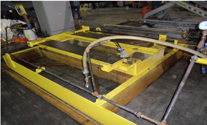
Figure 18: Example of Skid Mounted Equipment
