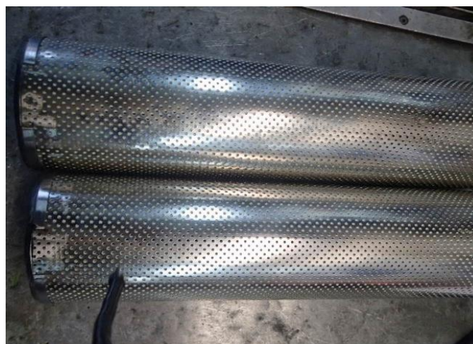
Figure 4: "New" LO Filters with protective plating.
