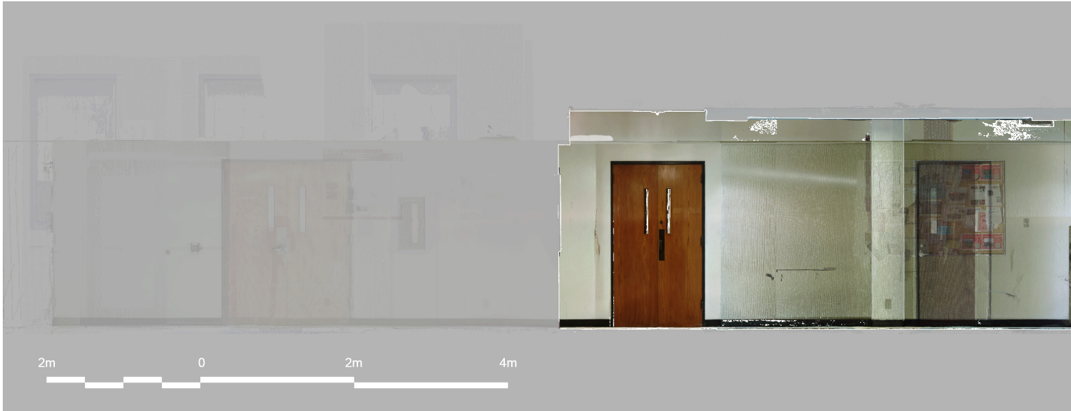
Figure 10. Transverse Section (Northwest-Southeast Axis, looking Northeast). Orthophoto of point cloud export from FARO Scene.
