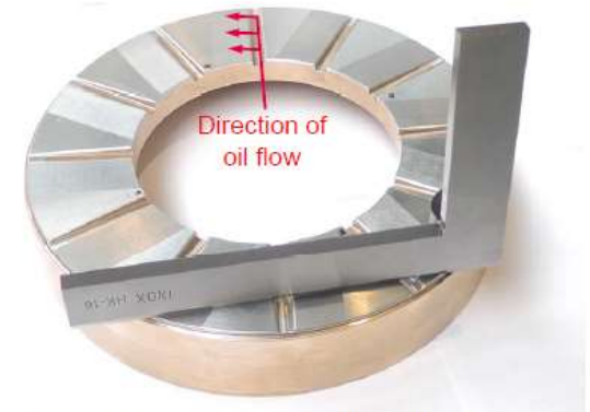
Picture 1: thrust bearing male rotor overview
