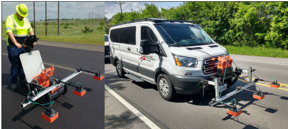
Figure 7. GPR Density Profiler. Reprinted from (9).
