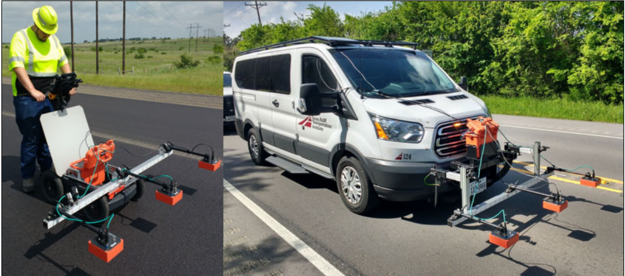
Figure 2. GSSI PaveScan Rolling Density Meter using GPR Technology. Reprinted from (9).
