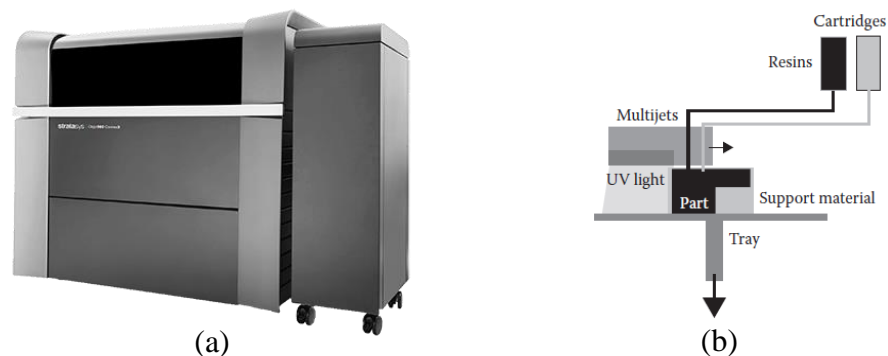
Figure 2. (a) The Connex3 Objet500 from Stratasys.com. This production-quality material jetting machine offers a build size of 490×390×200 mm, multiple material options, and layers as thin as 16 \mu\text{m} . (b) A diagram of the material jetting process [2].
