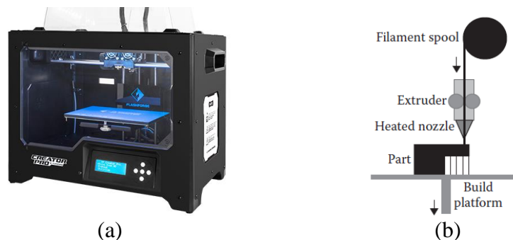
Figure 1. (a) The Creator Pro machine from flashforge.com. This FDM machine features a build volume of 227 \times 148 \times 150 mm, two extruders, and produces polymer parts with a minimum layer thickness of 0.1 mm. (b) A diagram of the FDM process [2].
