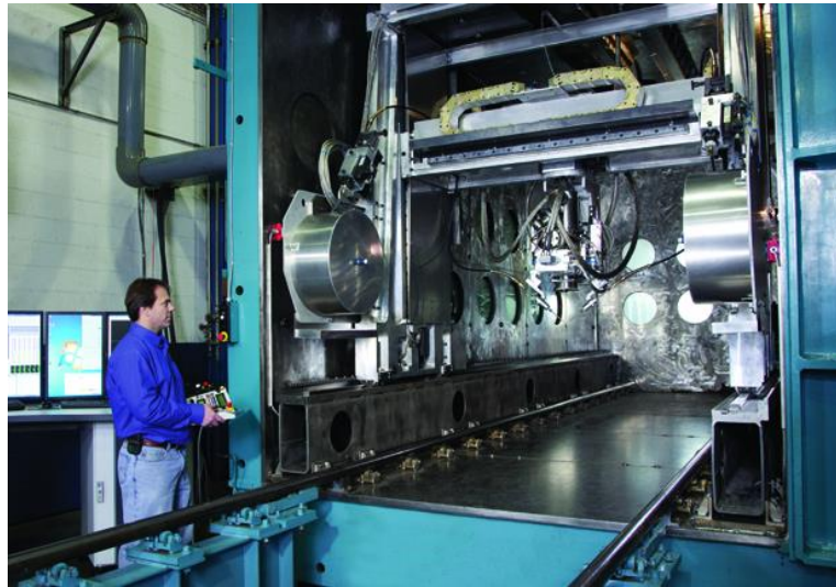
Figure 9. The EBAM 300 machine by Sciaky Incorporated. This machine uses electron beam additive manufacturing (EBAM) technology to create high-strength metal parts. It is claimed to be the largest 3D printer for metal parts that is fit for industrial and commercial use [14].
