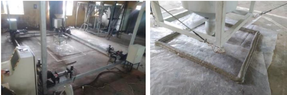
Figure 17. A recent example of a large-scale CSR for concrete FDM. The test path is a square with the side length of 0.8 m [55].
