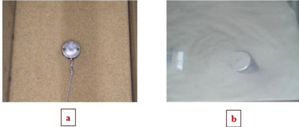
Figure 3.22: (a) A model caisson anchor and the mooring line connection. (b) a failed caisson anchor model. Reprinted from [Bang et al. 2011]
