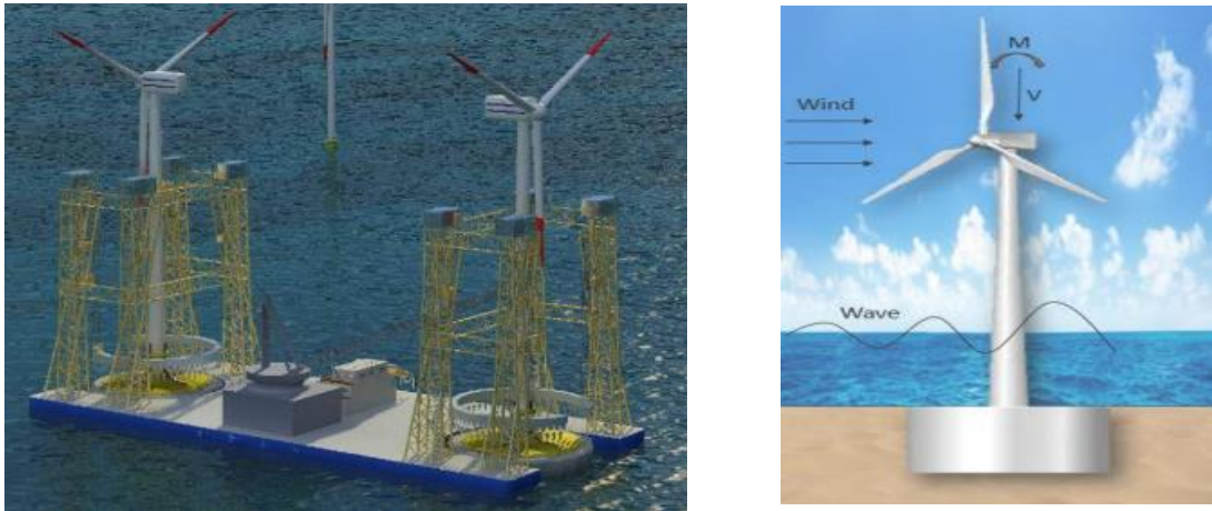
Figure 5.1: An offshore wind turbine with a monopod bucket foundation. Reprinted from [Achmus et al. ,2013]
