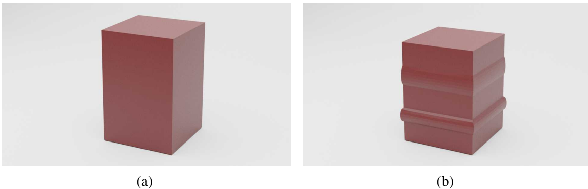
Figure 4.5: HETERO scene that divides a vertical bar mesh into layers of alternating material stiffness. Reprinted from [13].
