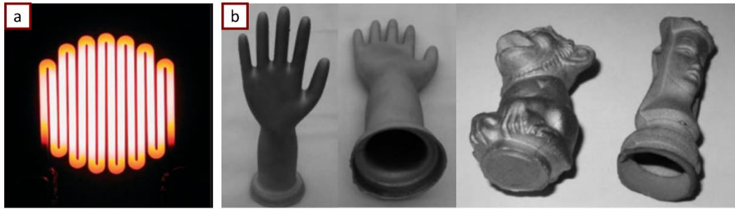
Figure 1-4 (a) \text{Ti}_2\text{AlC} -based heating element at 1450 °C in air; (b) Articles made by MAX phases. Images were adapted from [5].
