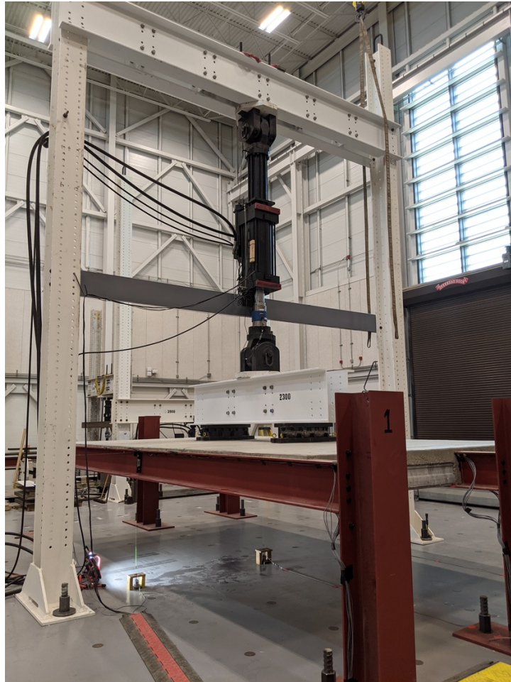
Figure 4.21: Actuator loading configuration (Photo by Matthew Yarnold)
