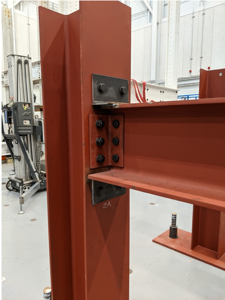
Figure 4.11: Fixed beam-to-column connection (Photo by Matthew Yarnold)
