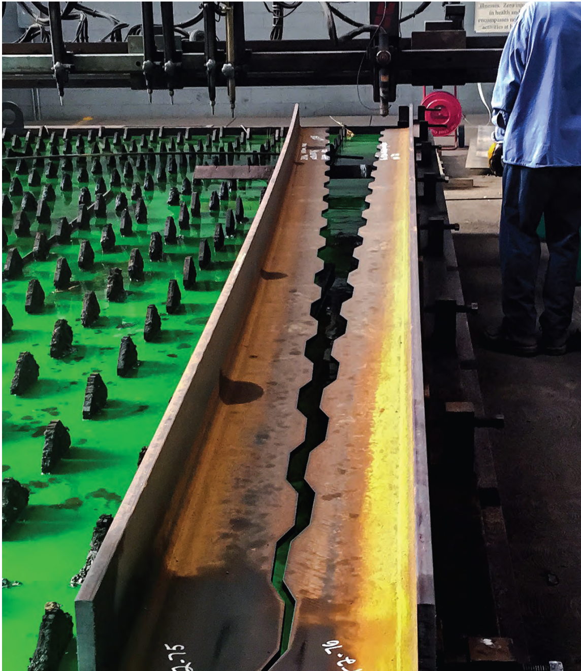
Figure 3.2: Castellated pattern cut to make D-BEAM® girder [13]
