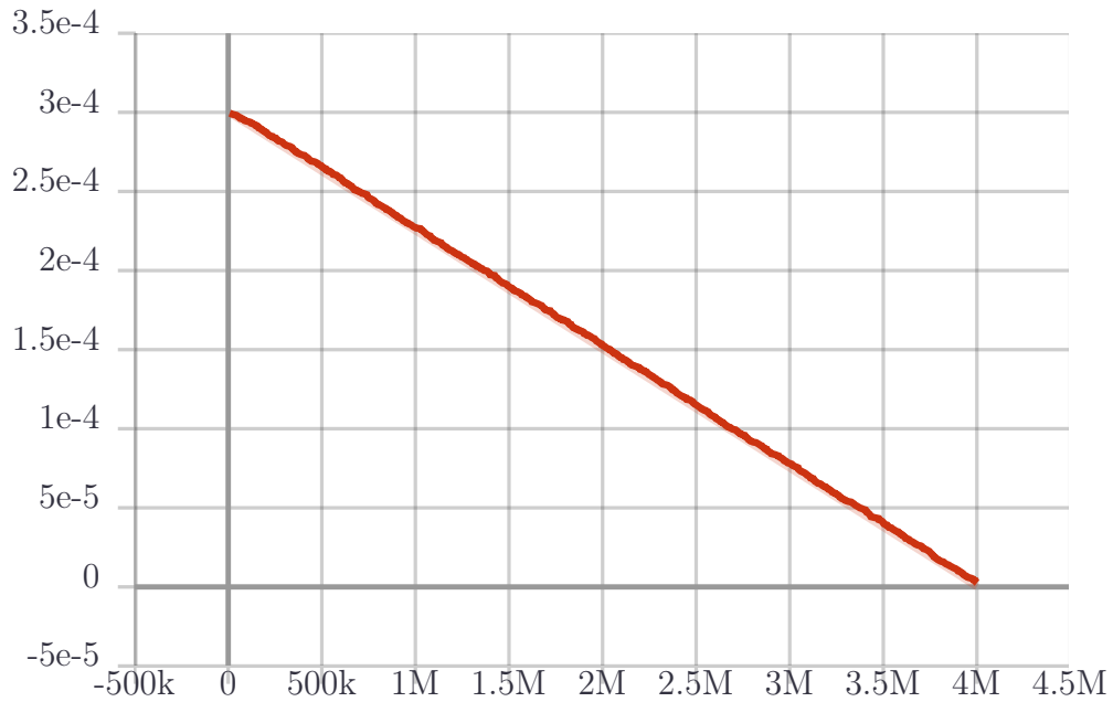
Figure 5.13: Stage 4: Learning rate (vertical axis) in each episode (horizontal axis) shown to be starting at the rate setup in PPO configuration and is gradually decreased as the updates need to be less frequent
