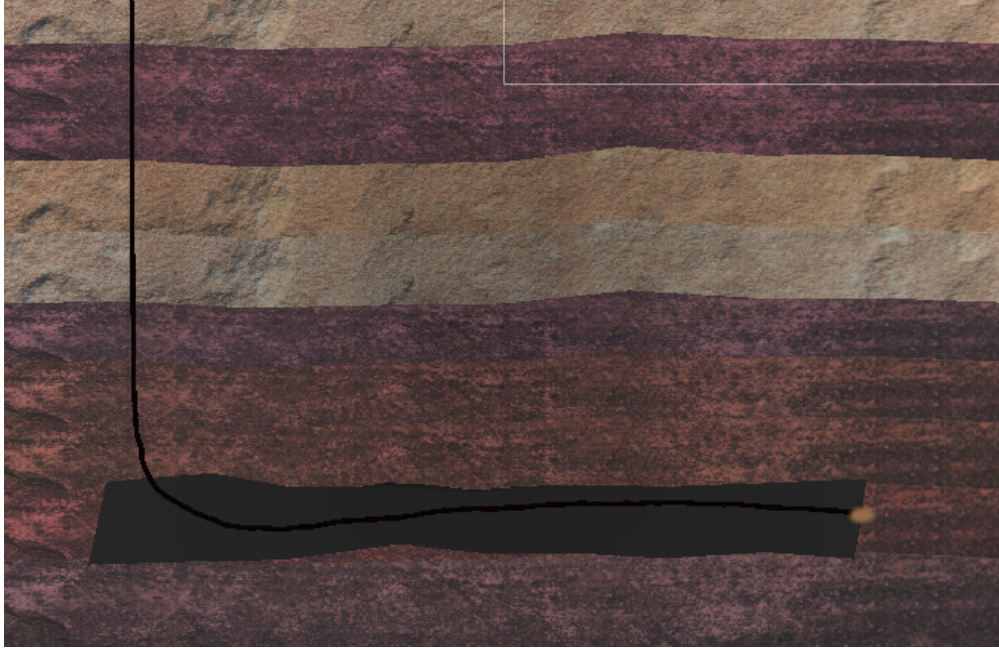
Figure 5.9: Model trained on the setup described in Stage 4 - shows the model is tuned and achieves the objectives of drilling through target zone maximizing exposure and minimizing tortuosities
