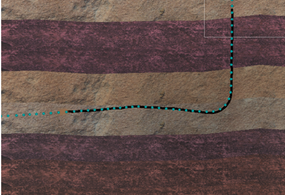
Figure 4.9: Model learned to accurately follow trajectory by slowing down at high build sections after the action space is expanded to include speed control
