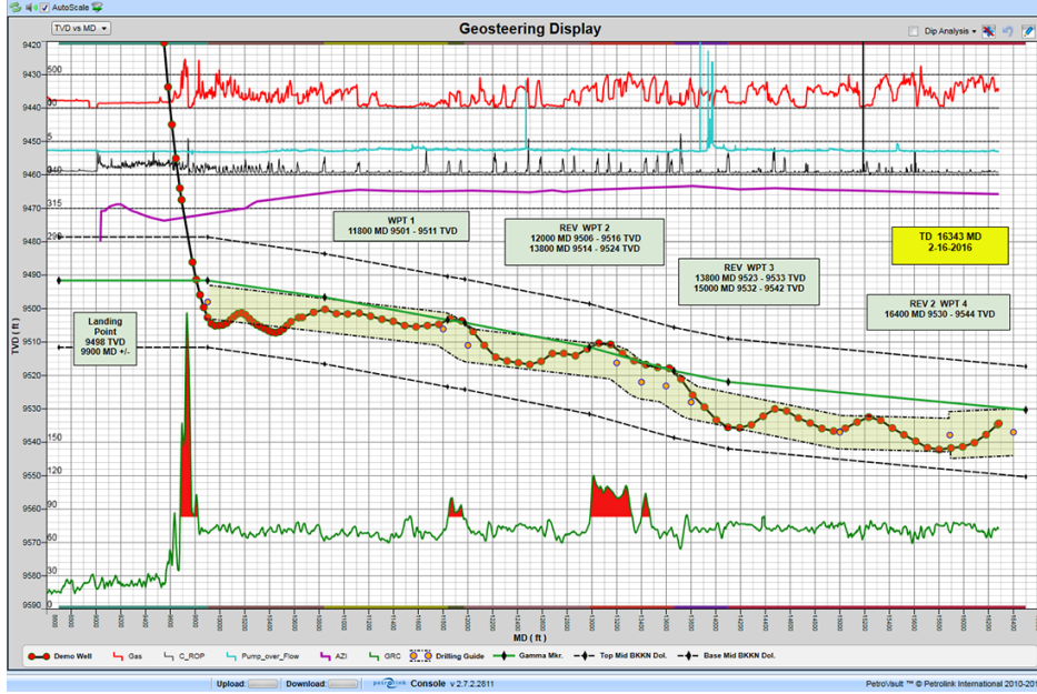
Figure 5.5: Snapshot of Real-time Geosteering operation monitoring highlighting the tortuous wellpath (red curve represents the actual trajectory drilled and the dots on the curve are survey points) in the target formation (represented as yellow strip in the center). ( Source: Petrolink )
