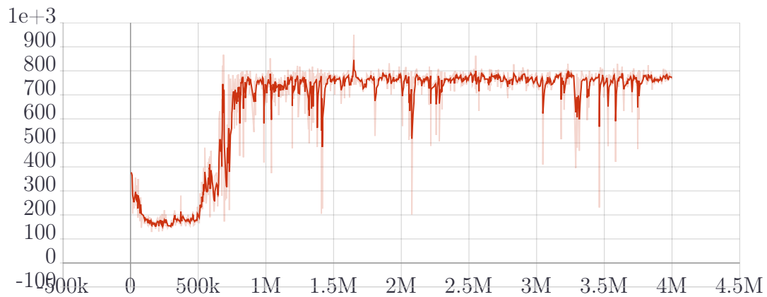
Figure 5.12: Stage 4: Length (vertical axis) of each episode (horizontal axis) are seen to be low in the early stage while exploring and to be large and consistent as the agent learned to take higher number of correct actions
