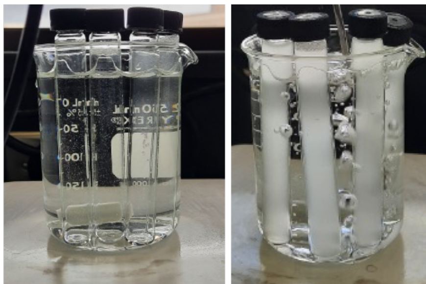
Figure 22 – Cloud point measurement for temperature below 200° F, showing before cloud point (left) and after cloud point (right).
