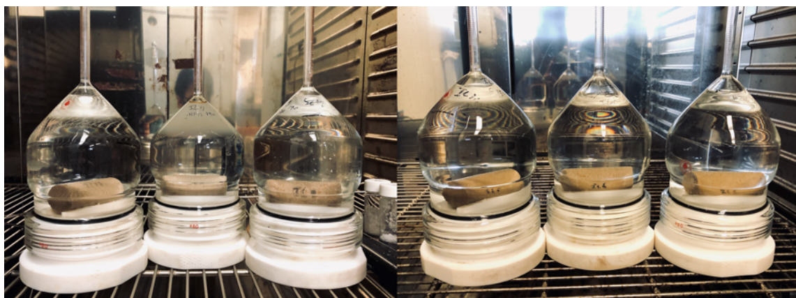
Figure 24 – Custom Amott cells, “The Taj”, to perform spontaneous imbibition experiments.
