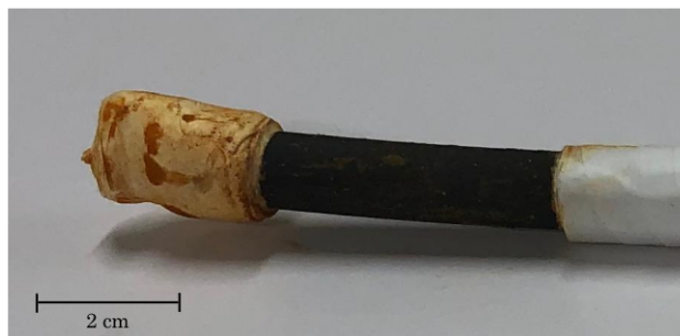
(d) As-Received ASTM A 416 wire tested in a corrosive environment (pH=7).
