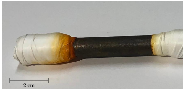
(c) Uncoated ASTM A 416 wire tested in an acidic environment (pH=3.8).
