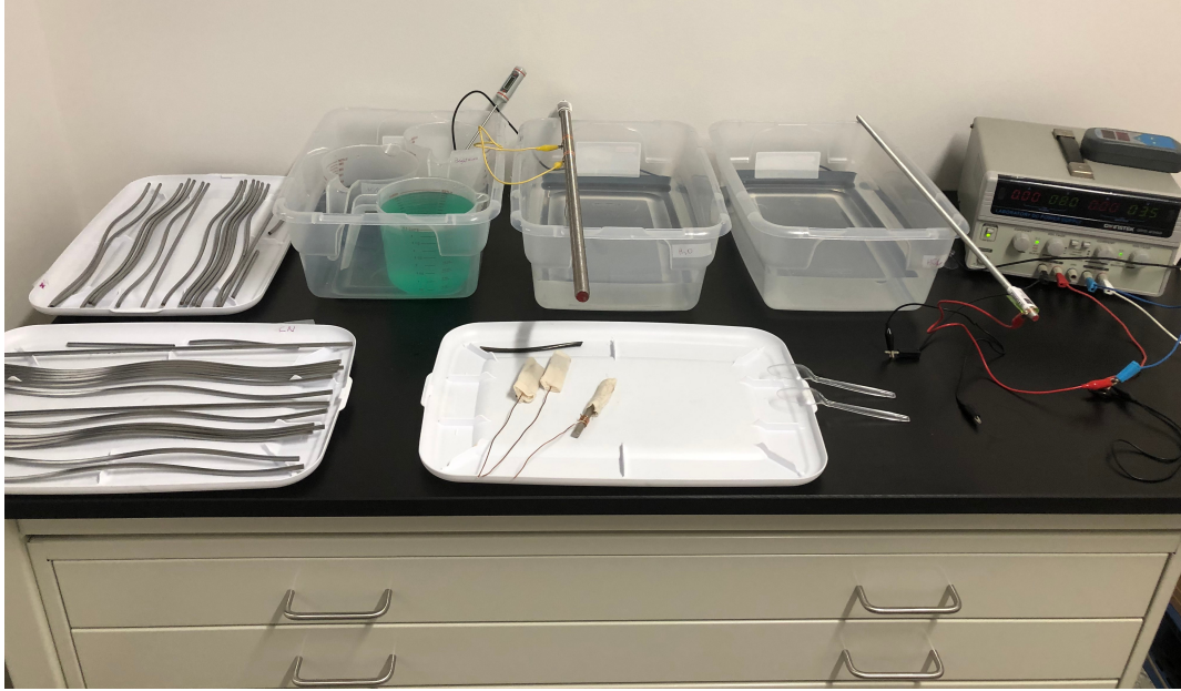
Figure 3.3: Apparatus and materials used for metallic coating on steel wires.
