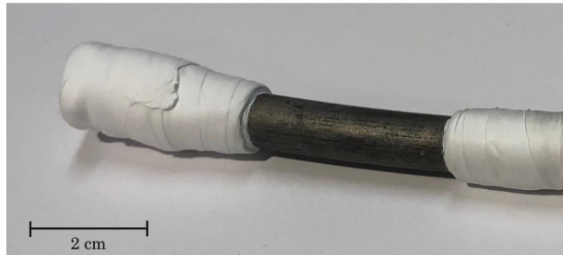
(c) Ni/Co coated wire protected in corrosive environment (pH=7).
