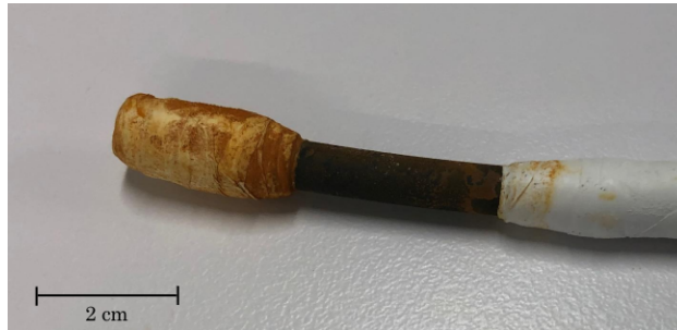
(e) Uncoated ASTM A 416 wire tested in a corrosive environment (pH=7).
