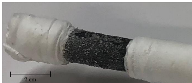
(l) Zn/Ni coated wire placed in a simulated pore solution for two days then exposed to air.
