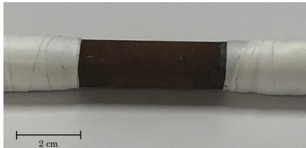
(g) Zn/Ni coated wire protected with impressed current. The potential limit to protect the sample was not achieved, causing the zinc coated layer to break off and develop uniform pits on the surface of the substrate. Pits were small and it was difficult to see with an unaided eye. After the sample was left at room temperature for a day, the uniform pits propagated throughout the surface and caused uniform corrosion.
