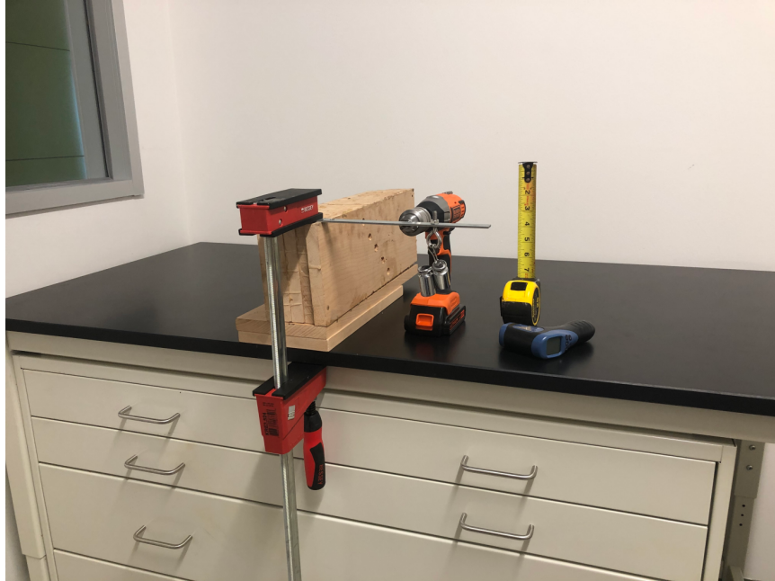
Figure 8.1: Sliding process that was completed with a 30 \times 2 cm [ 12 \times 3/4 in] galvanized cantilever beam.
