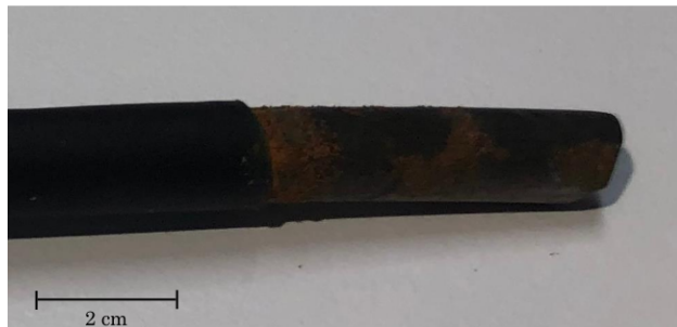
(d) Ni/Co coated wire exposed to corrosive environment (pH=7).
