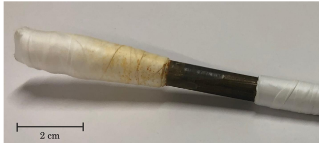
(a) As-Received ASTM A 416 wire tested in a corrosive environment (pH=7).
