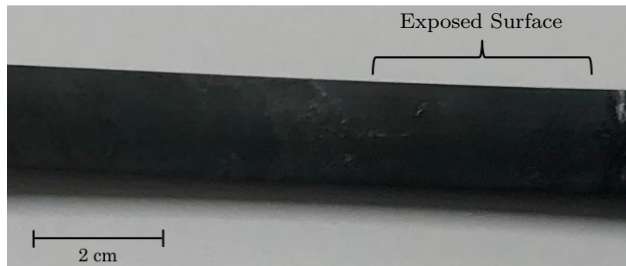
(d) Zn/Ni coated wire tested in a corrosive environment (pH=7).
