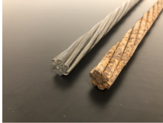
Figure 3.1: Comparison between intact and corroded ASTM A 416 strands. The corroded steel strand was left outside for more than 3 years and were exposed to air and moisture.
