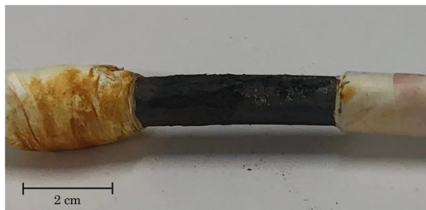
(b) As-Received ASTM A 416 wire tested in an acidic environment (pH=3.8).
