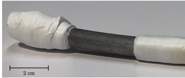
(a) Uncoated steel wire protected in corrosive environment (pH=7).
