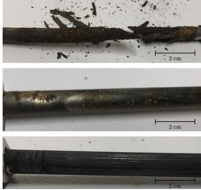
Figure 7.5: As-received specimen as well as nickel-cobalt and zinc-nickel coated wires a month after the embrittlement test, from top to bottom respectively.
