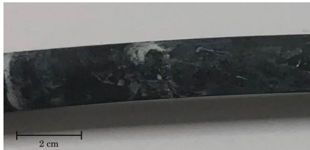
(k) Zn/Ni coated wire tested in a simulated pore environment (pH=12).
