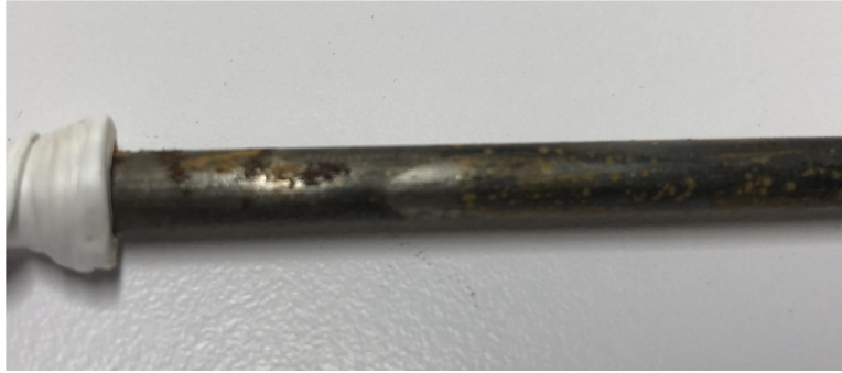
Figure 2.11: Pitting corrosion. Corrosive agents attacked ASTM A 416 steel coated with nickel-cobalt alloy and caused the formation of corrosion pits.
