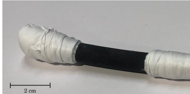
(e) Zn/Ni coated wire protected in corrosive environment (pH=7).
