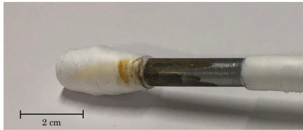
(b) Uncoated ASTM A 416 wire tested in a corrosive environment (pH=7).
