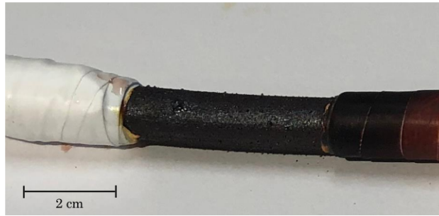
(a) As-Received ASTM A 416 wire tested in an acidic environment (pH=3.8).
