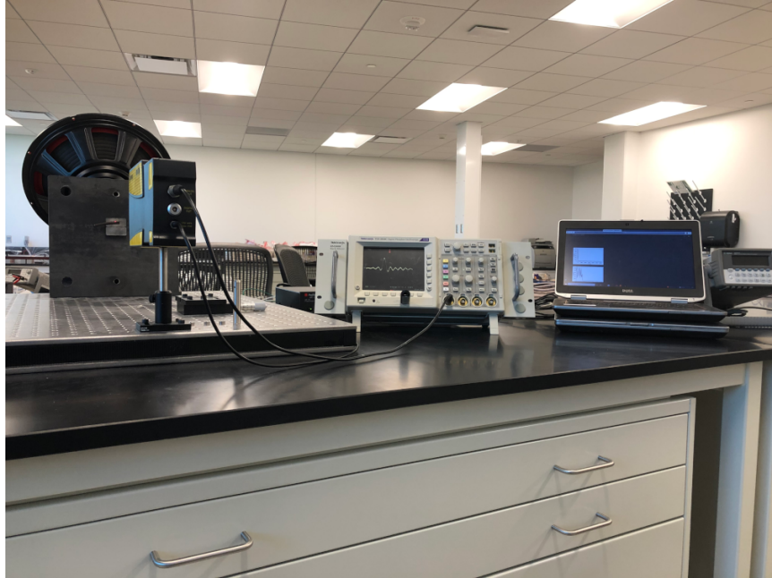
Figure 8.2: Oscilloscope visualization of the signals from the optical laser where a python script saved time domain signals in CSV files, simultaneously.
