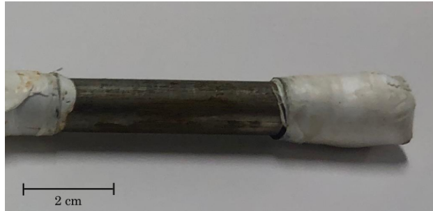
(i) Ni/Co coated wire tested in a simulated pore environment (pH=12).
