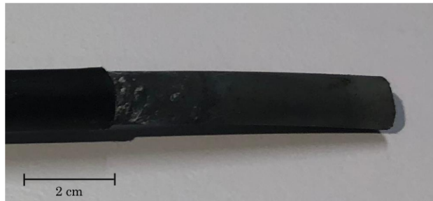
(f) Zn/Ni coated wire exposed to corrosive environment (pH=7).
