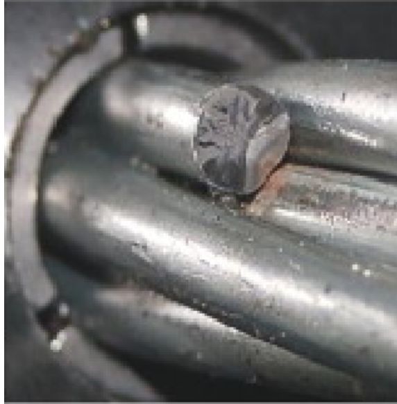
Figure 2.13: Rupture of steel wire due to fretting fatigue, reprinted from (Winkler et al., 2015) with permission.
