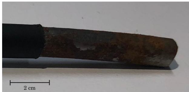
(b) Uncoated steel wire exposed to corrosive environment (pH=7).
