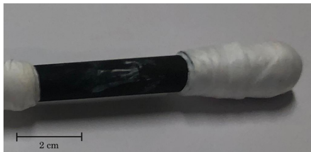
(j) Zn/Ni coated wire tested in a corrosive environment (pH=7).
