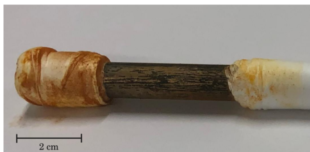
(h) Ni/Co coated wire tested in a corrosive environment (pH=7).
