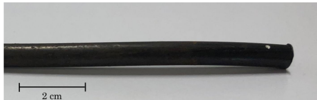
(g) As-Received ASTM A 416 wire—scale and injurious defect.
