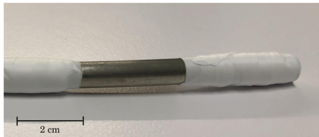
(c) Ni/Co coated wire tested in a corrosive environment (pH=7).
