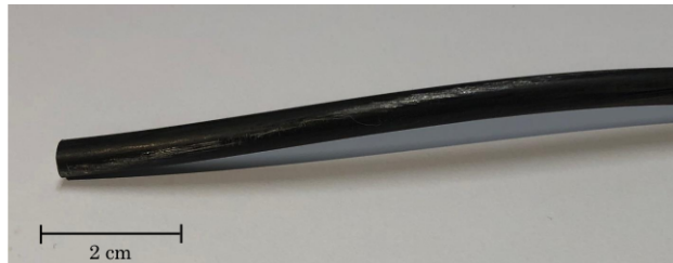
(f) As-Received ASTM A 416 wire—abrasive wear damage.
