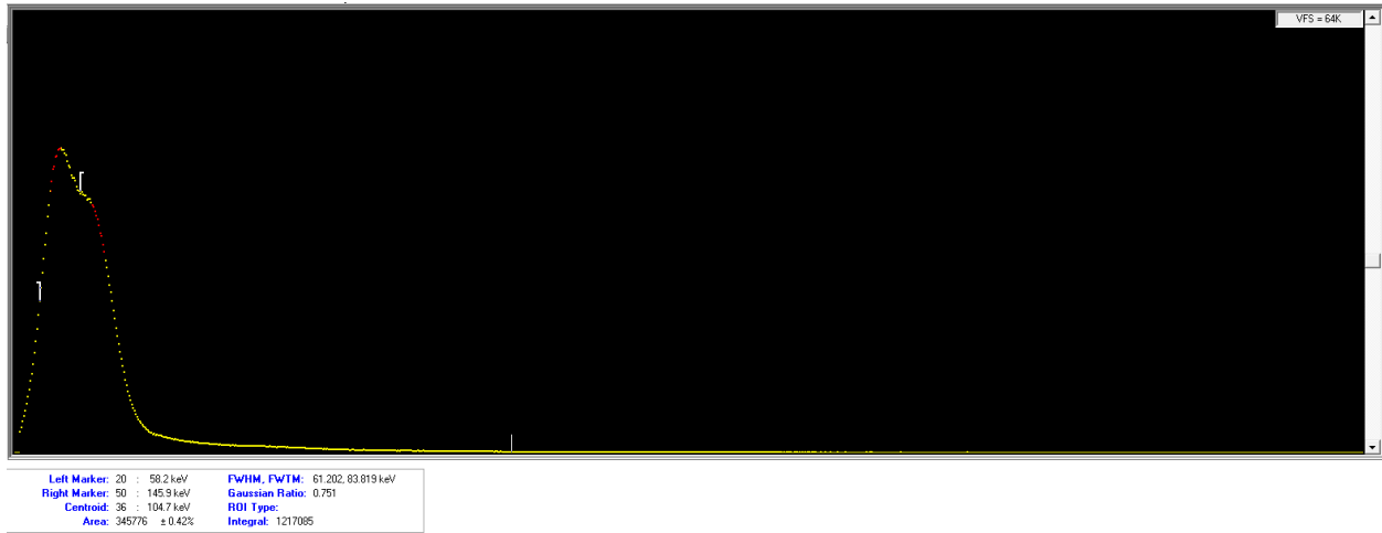
Figure N.5. Genie spectrum for HEU shielded to 50% intensity at a 30% resolution. The source configuration was not identified, even with a 0.1 confidence level.
