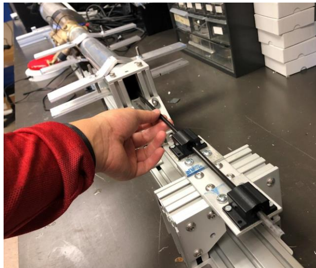
<Inserted carbon rod into the air cannon barrel front outlet>
