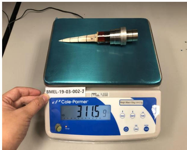
<Example of Measuring Projectile Mount Assembly Weight>
