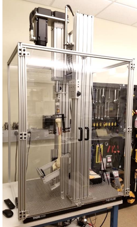
Figure 7 - The RTS in uniaxial mode with a linear actuator attached to the framework
