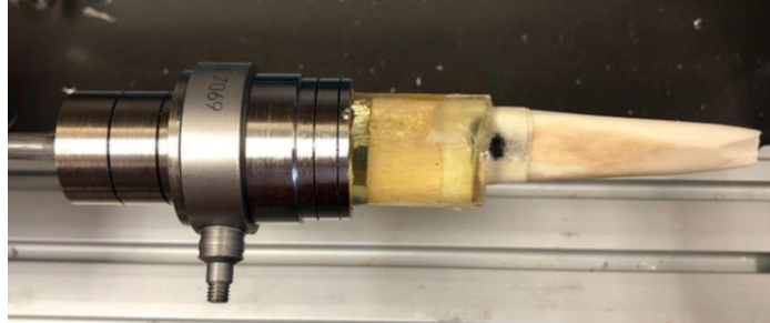
< Example of 'FIX-0075 Projectile Tip Mount of Air Cannon' assembly >
