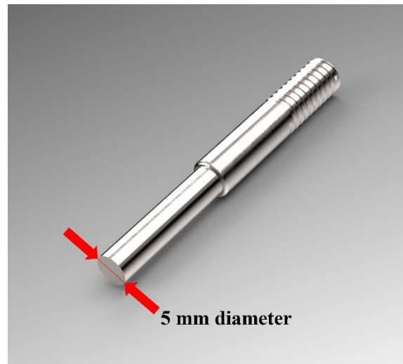
Figure 49 - Push-out indenter with 5 mm diameter (flat-bottomed)
