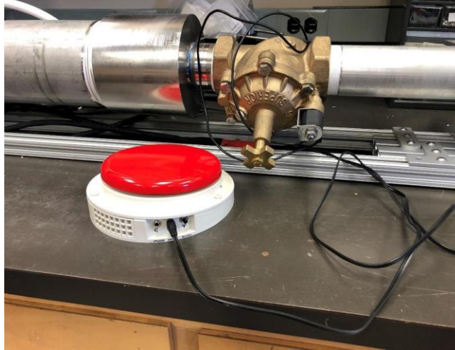
<Connected Push button switch (red) with solenoid valve of Air cannon (FIX-0073)>
