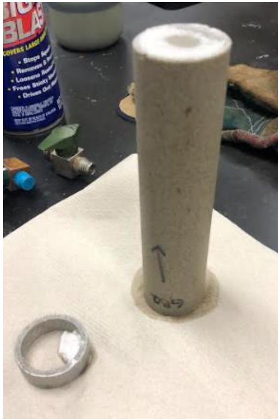
Figure III- 15a Sandstone core after exposure to micronized barite (5 \mu\text{m} ) water-based drilling fluid
