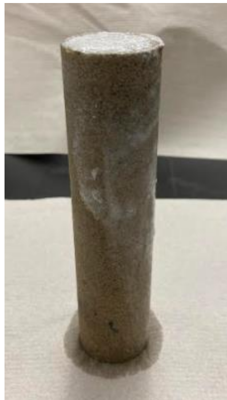
Figure III- 14a Sandstone core after exposure to micronized barite (2 \mu\text{m} ) water-based drilling fluid
