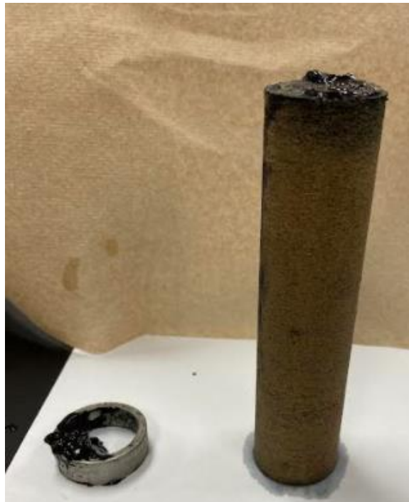
Figure III- 16a Sandstone core after exposure to micronized ilmenite (5 \mu\text{m} ) water-based drilling fluid
