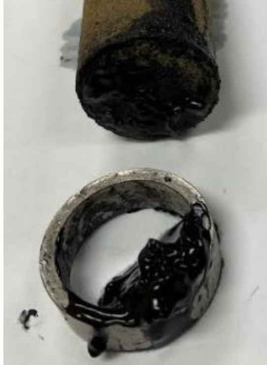
Figure III-16b Micronized ilmenite (5 \mu\text{m} ) filter cake formed across the face of the sandstone core
