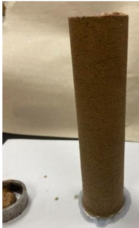
Figure III- 13a Sandstone core after exposure to API barite water-based drilling fluid
