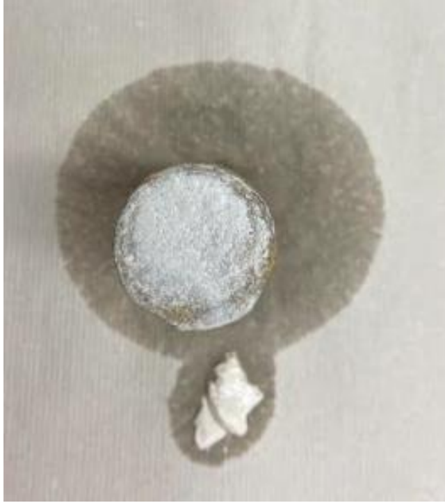
Figure III- 14b Micronized barite ( 2\ \mu\text{m} ) filter cake formed across the face of the sandstone core
