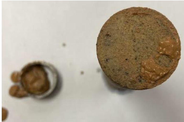
Figure III- 13b API barite-based filter-cake formed across the face of the sandstone core
