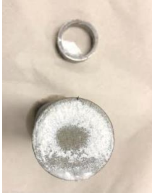
Figure III- 15b Micronized barite (5 \mu\text{m} ) filter cake formed across the face of the sandstone core
