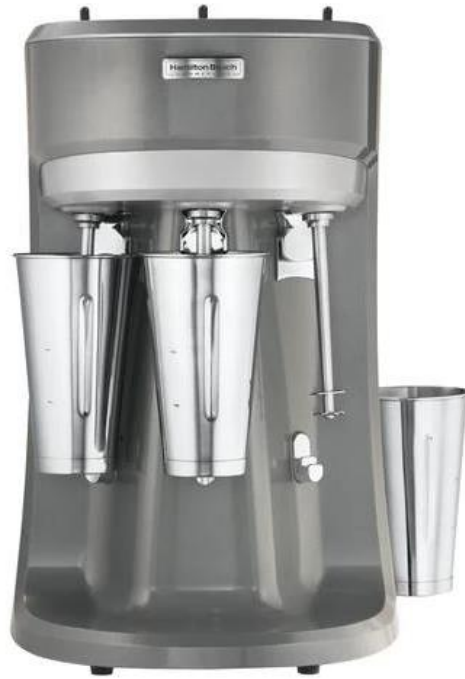
Figure II-1 Drilling fluid mixer
