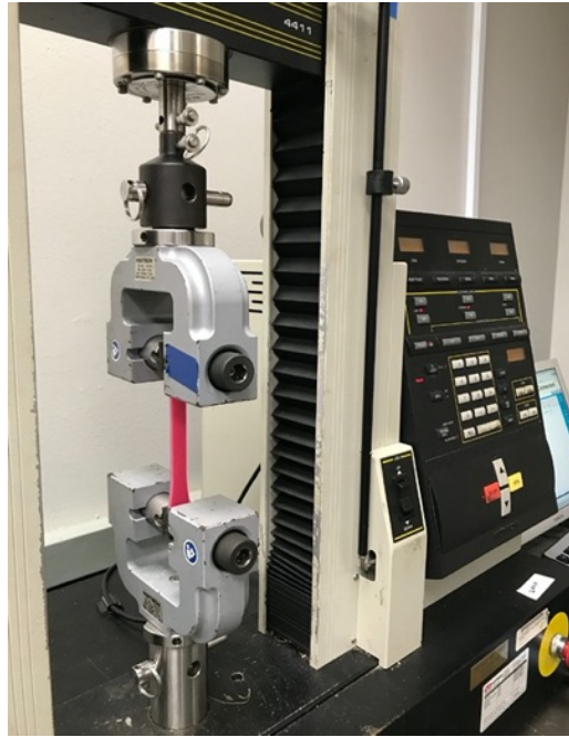
Figure 2.4 Instron 4411 tensile testing machine
