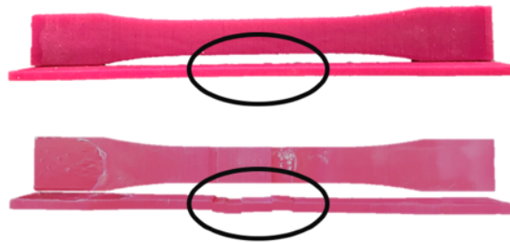
Figure 2.3 Printed sample without support parts (bottom), and printed sample with support parts (top)
