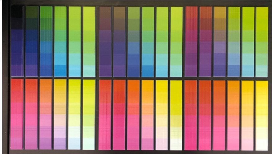
Figure 5.2 Printed 216 samples and their layout on the build platform.
