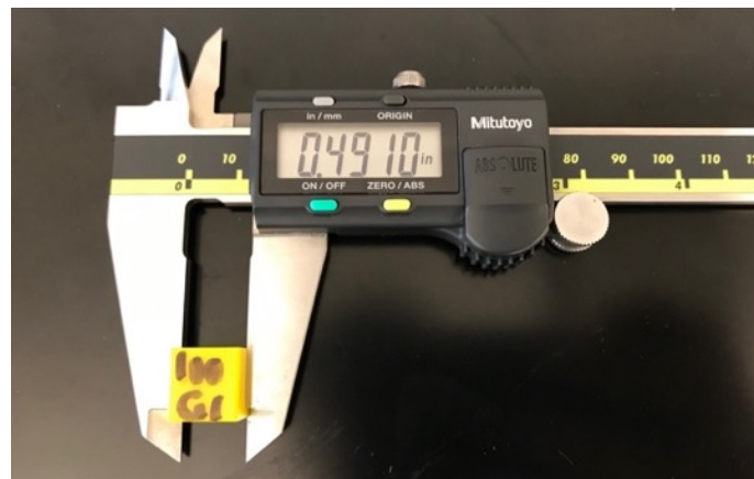
Figure 3.3 Dimensional measurement along the X axis for “100G1”
