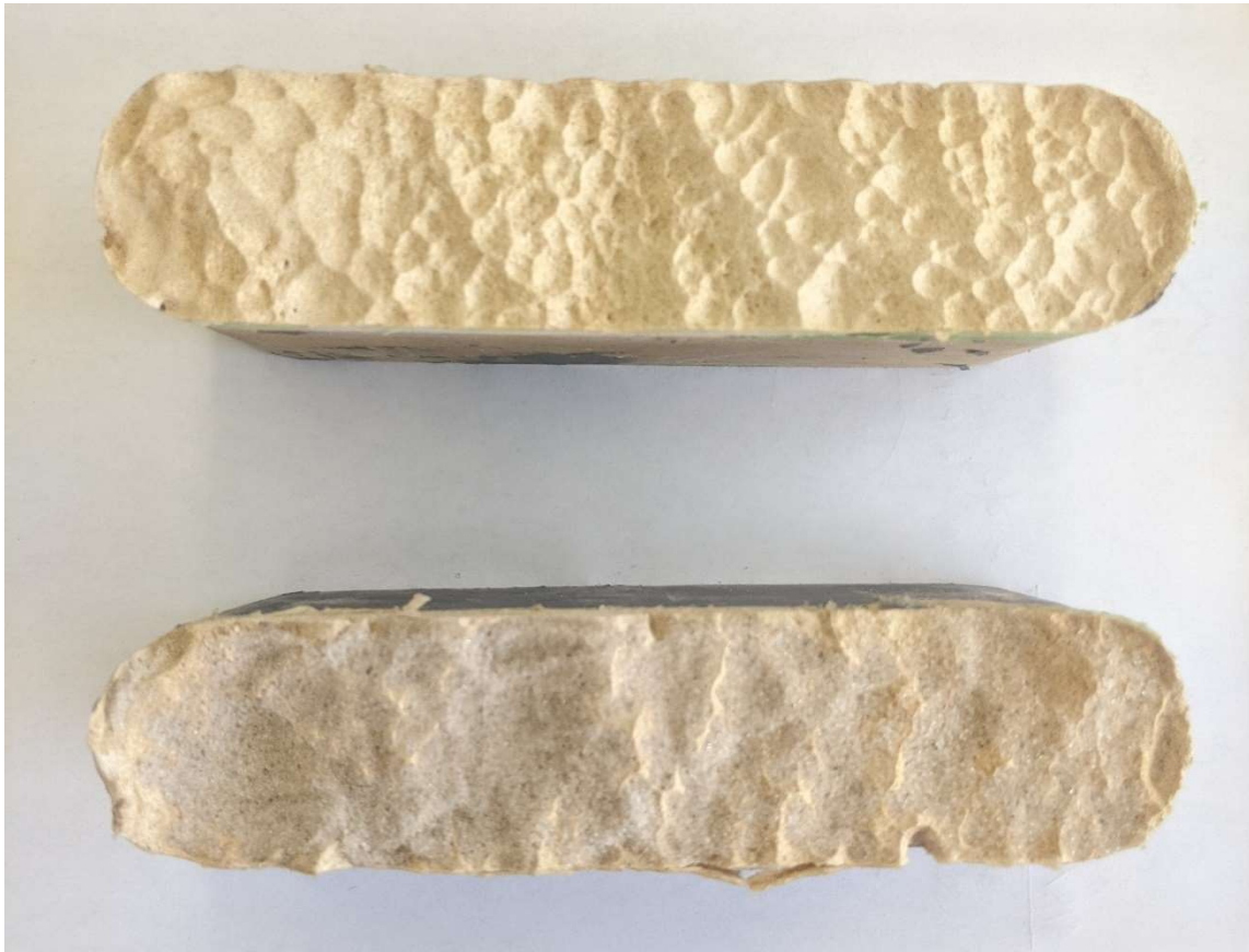
Figure 6: Proppant evenly distributed onto the bottom of the sample (the sample half at the bottom of the figure).
