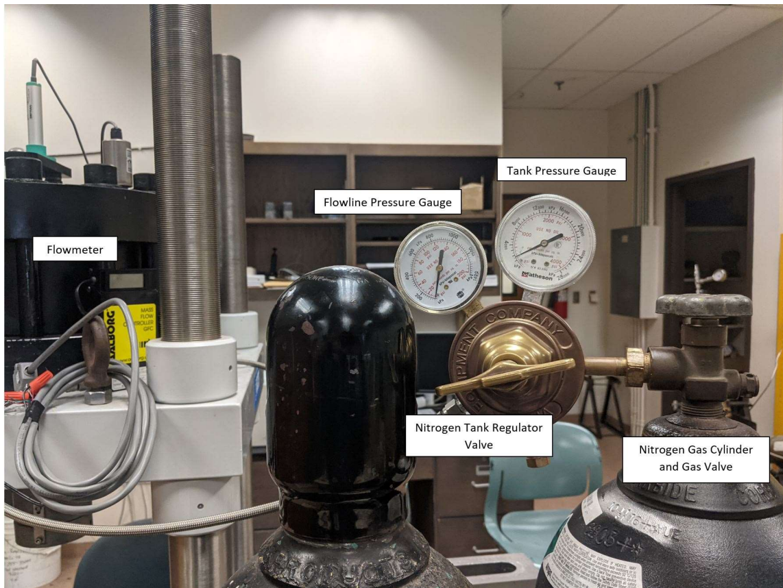
Figure 17: Experimental setup showing the gas cylinders and flow gauges.
