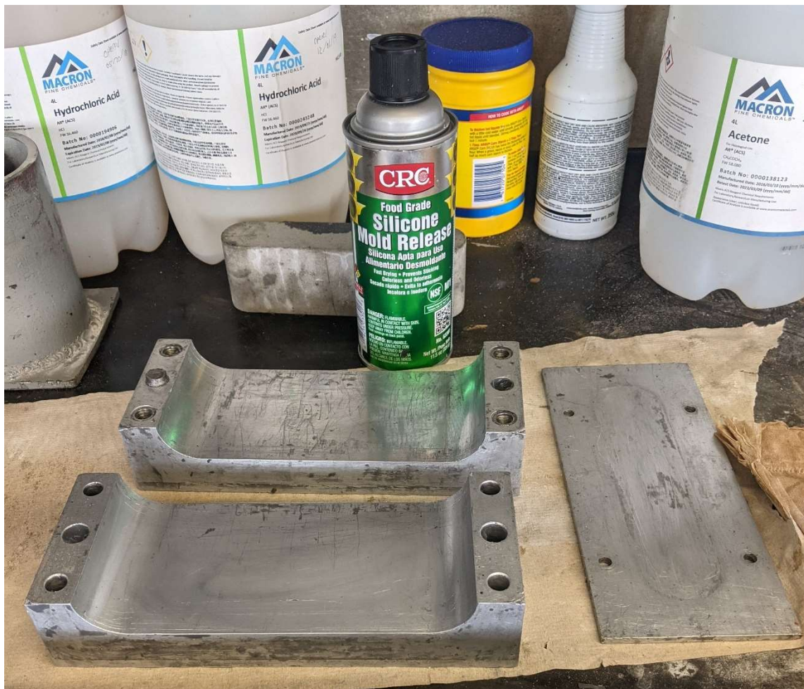
Figure 8: Sample mold and mold release spray under a fume hood.
