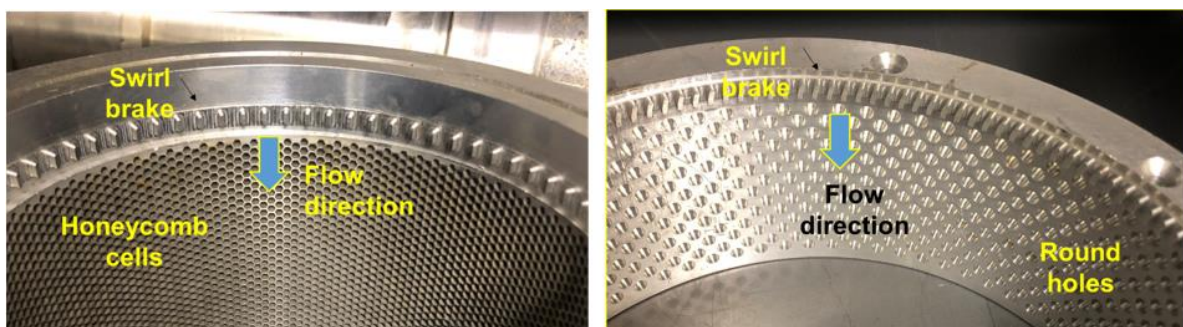
Figure 5 Photographs of a honeycomb seal and a hole-pattern seal, both with swirl brakes upstream of the seal entrance.
