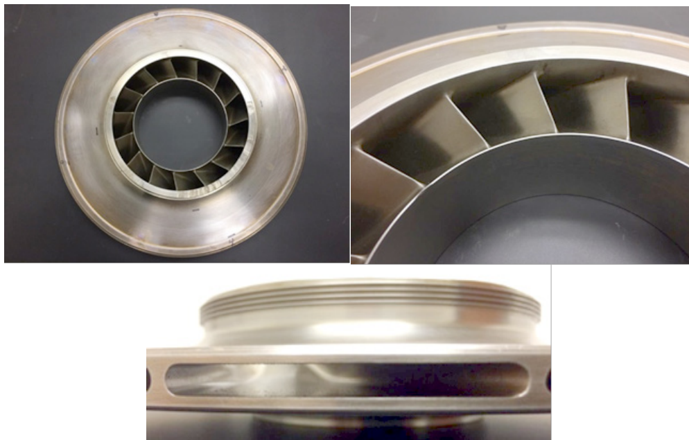
Figure 6. Images showing the EDM'd full impeller
