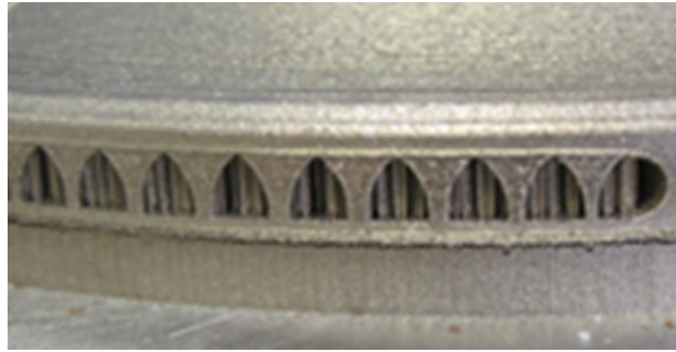
Figure 24. Image of the Full DMLS impeller as built on the baseplate
