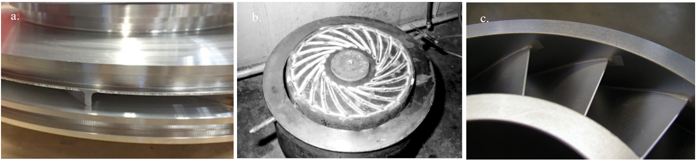
Figure 2. Examples of two piece impellers, including an impeller prepped for fillet welding (a.), a slot welded impeller in a fixture (b.), and an impeller brazed using foil and paste
