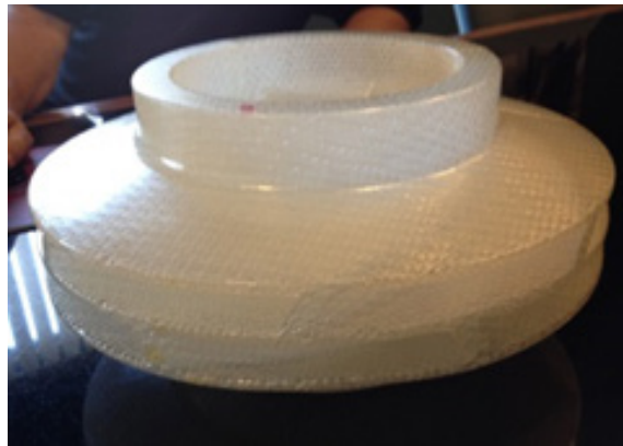
Figure 13. Photo of a QuickCast pattern of a double flow pump impeller
