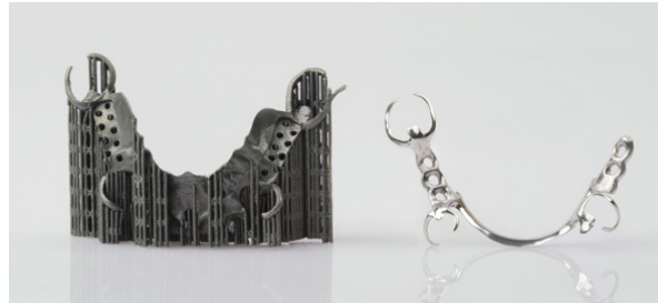
Figure 21. As printed (left) and finished dental apparatus (courtesy EOS)
