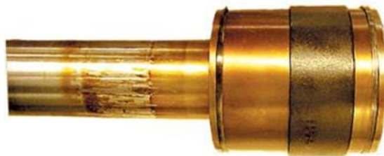
Figure 3: Varnish on an inlet guide vane valve. Reprinted from Fitch and Gebarin (2006). The varnish has a cured, shiny, golden-like appearance that cannot be wiped from the surface.
