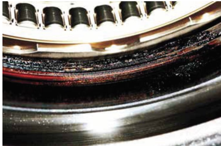
Figure 1: Sample of coke deposits. Reprinted from Exxon Mobil Corporation (2016).
