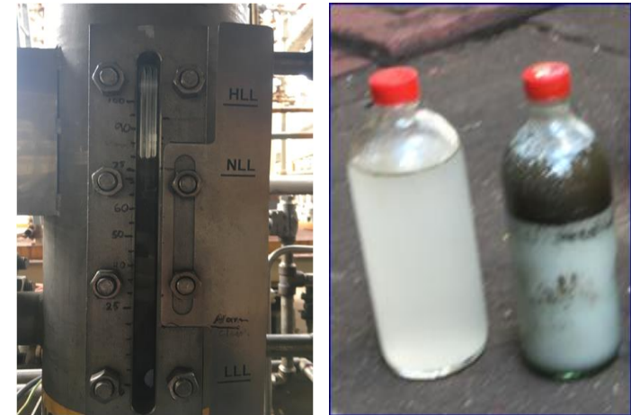
Figure: Sample of liquid in seal pot (flow reversal indication)
