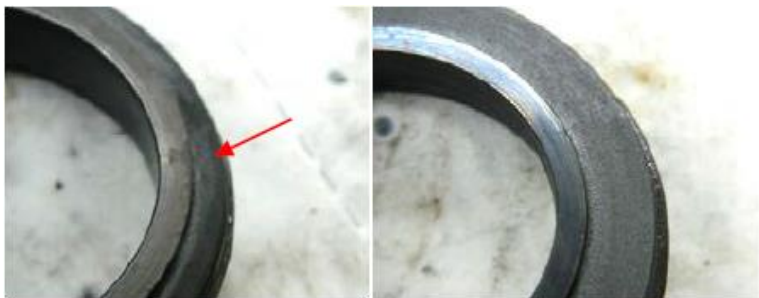
Figure: Seal face worn out and blistering
