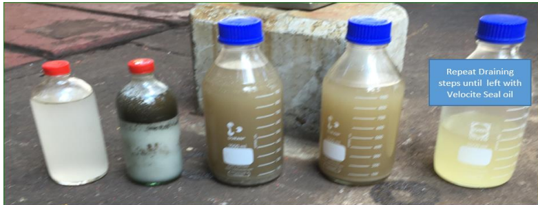
Figure: Series of draining performed to remove “milky” solution; after ~1month operation
