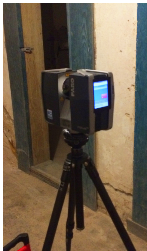
Figure 6: Riegl Scanner (above) Figure 7: FARO Scanner (below)
