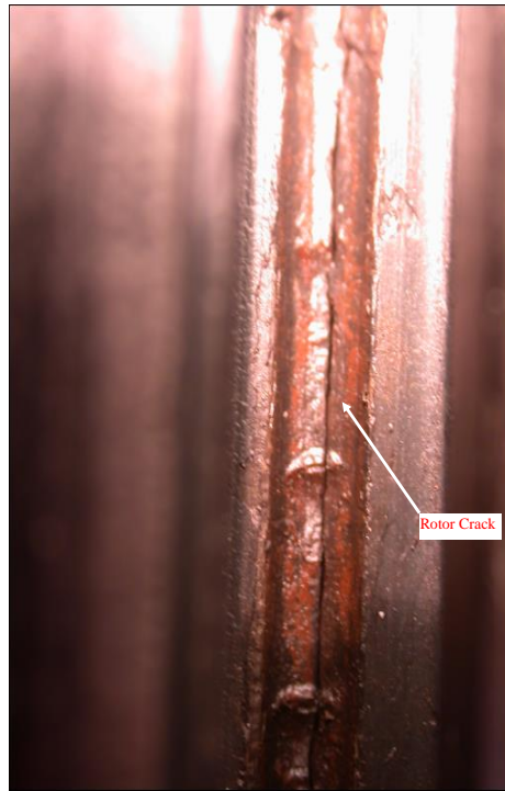
Fig. 18. The steam turbine rotor dovetail groove with circumferential crack
