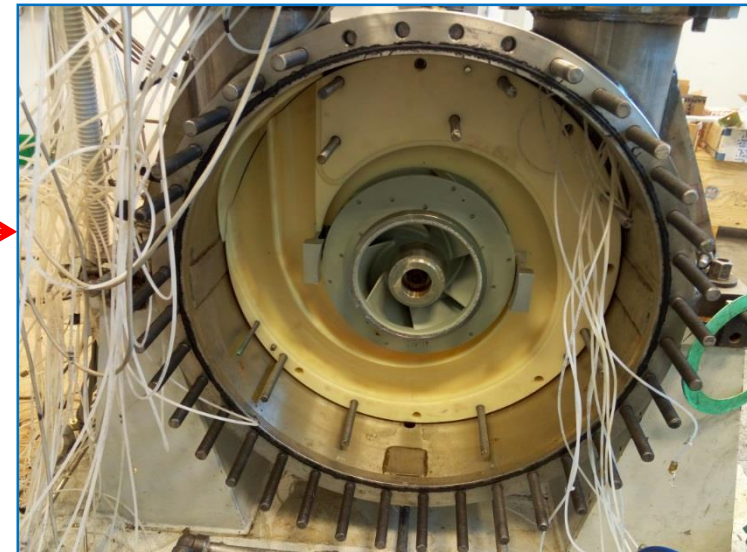
Figure 18 – Prototype With Impeller and Discharge Volute Assembled
