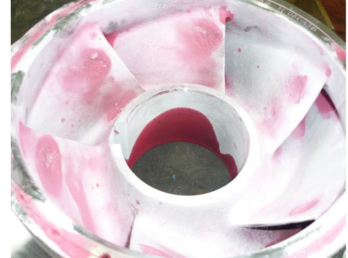
Figure 1 - Impeller Erosion at Suction Indication of Suction Recirculation
