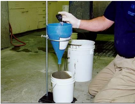
Figure 6: Measure the Time it takes for Grout to pass through the Flow Cone
