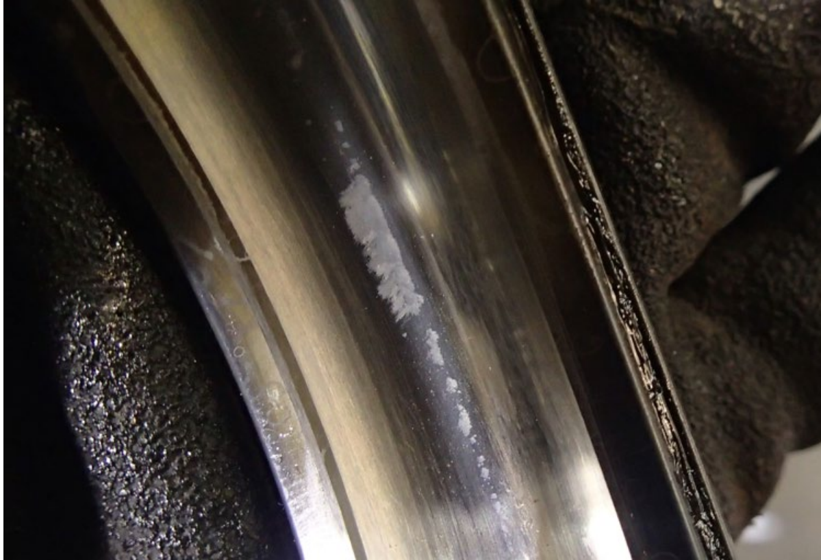
Figure 8: Bearing outer race damage.
