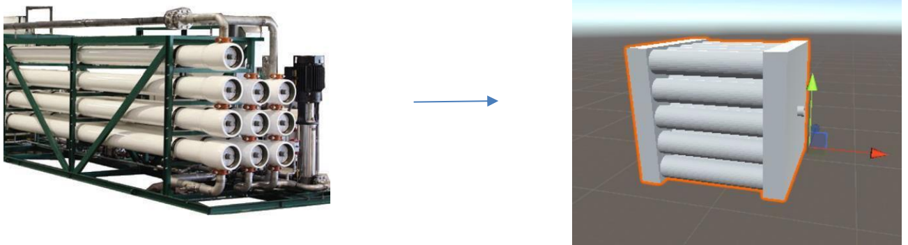
Figure 8: On the left, is the Reverse Osmosis Membrane (AMTEC, 2017) that desalinates the water using the process of reverse osmosis, and on the right is the recreated 3D model in SolidWorks
